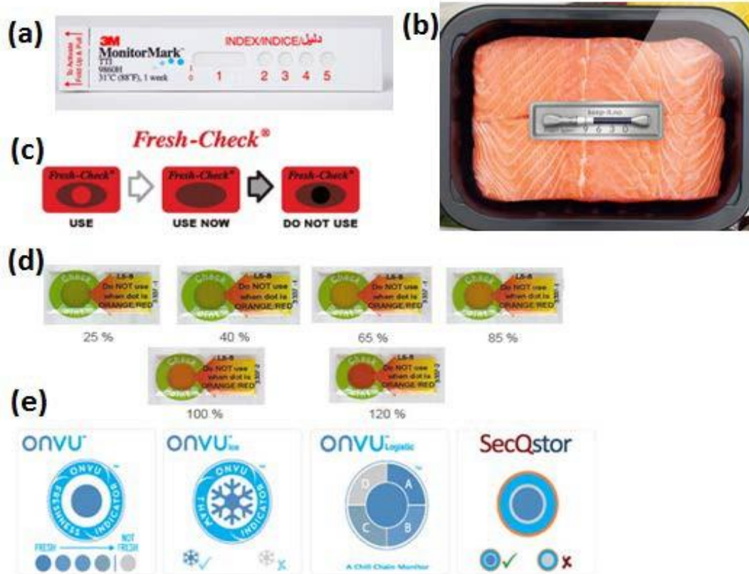
Fig.3. Examples of TTIs: (a) MonitorMark™, a self-adhesive label for monitoring thermal exposure of temperature-sensitive products during transportation and storage; (b) Keep-it, a TTI that predicts remaining shelf-life; (c) Fresh-Check®, a self-adhesive TTI specifically formulated to match the shelf life of the food products to which it is affixed; (d) VITSAB, a customised TTI label, such as the L5-8 Seafood label, which provides consumers with a full history of customised cold chain information; (e) OnVu™, a tailored TTI calibrated for the different spoilage behaviour of various foods and beverages, which is designed to be highly accurate and consistent in recording and displaying the freshness of the products, based on their time and temperature histories.
