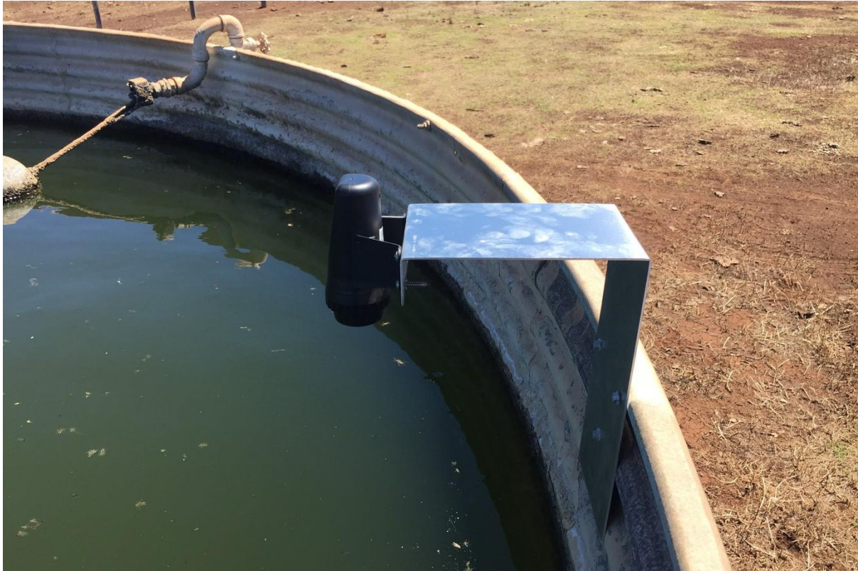
Figure 3: Waterwatch LS1-R Horizontal Mount Radar Level Sensor
