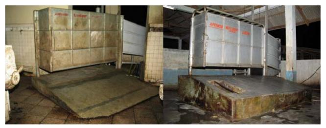
Figure 01 Mark I restraining boxes showing lower plinth height (left figure) and modified box with raised plinth (right figure)
