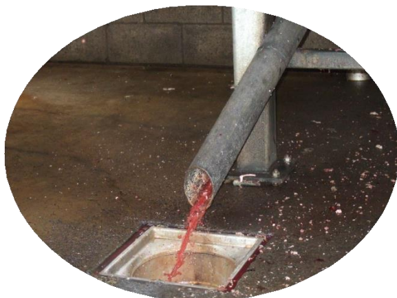
Photo 4. Raw material screw drain – although rich in blood, the low and intermittent flow makes it of little overall consequence.
