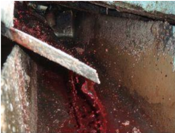
Photo 1. Raw material bin drainage – a very strong waste stream
