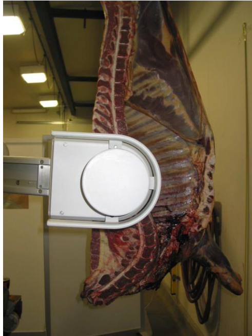
Figure 29: Tracking the vertebrae, looking for the correct rib
