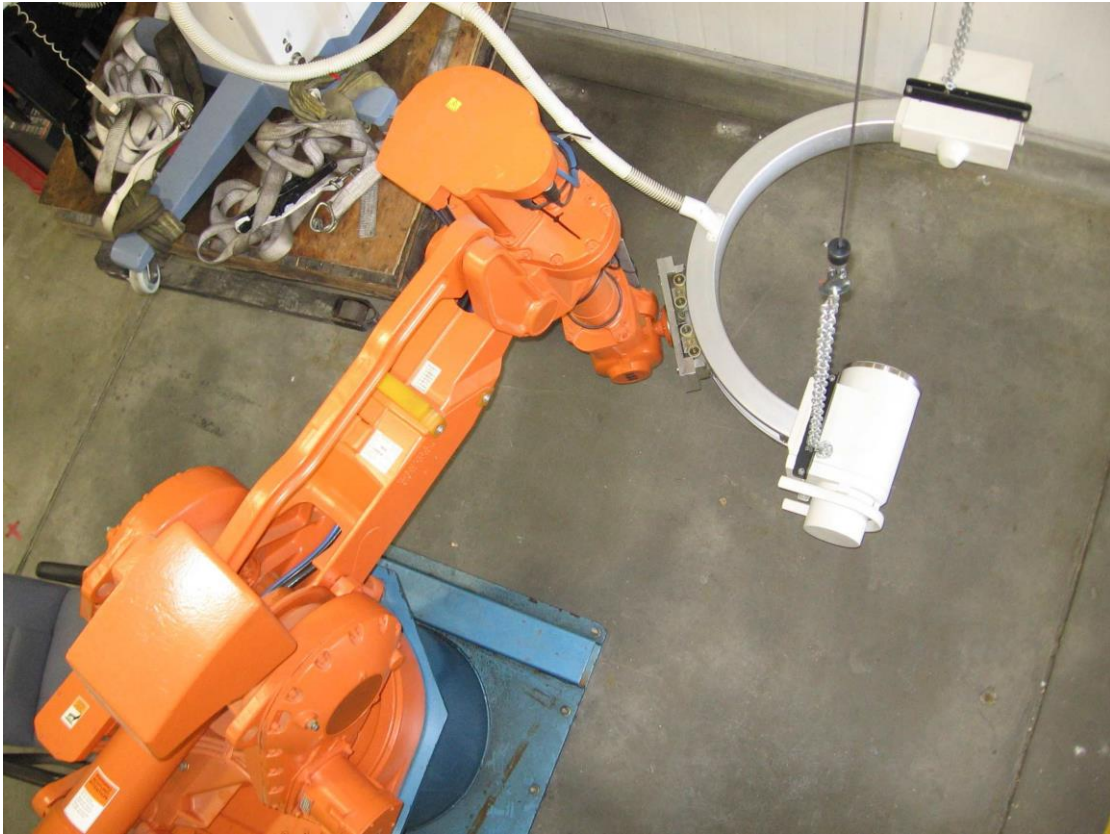
Figure 2 X-ray C-arm - robot mounting arrangement from above
