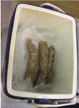
Figure 4: Control samples, wrapped in glad wrap and packaging tape, placed in an esky, for transport to the CSIRO-Coopers Plains laboratory
