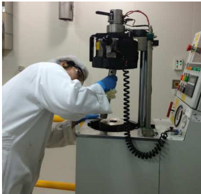
Figure 5: Samples being subjected to high pressure processing, after being transported to the CSIRO-Coopers Plains laboratory
