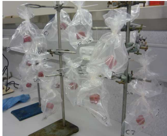
Figure 3: The hanging method for measuring drip loss of whole muscle.
