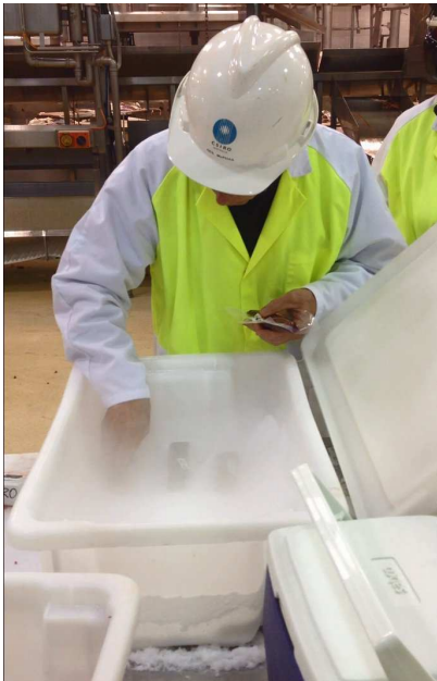
Figure 5: Samples being subjected to very fast chilling, using dry ice
