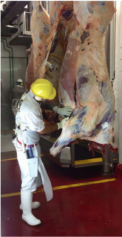
Figure 1: The brisket being hot-boned from a beef carcass
