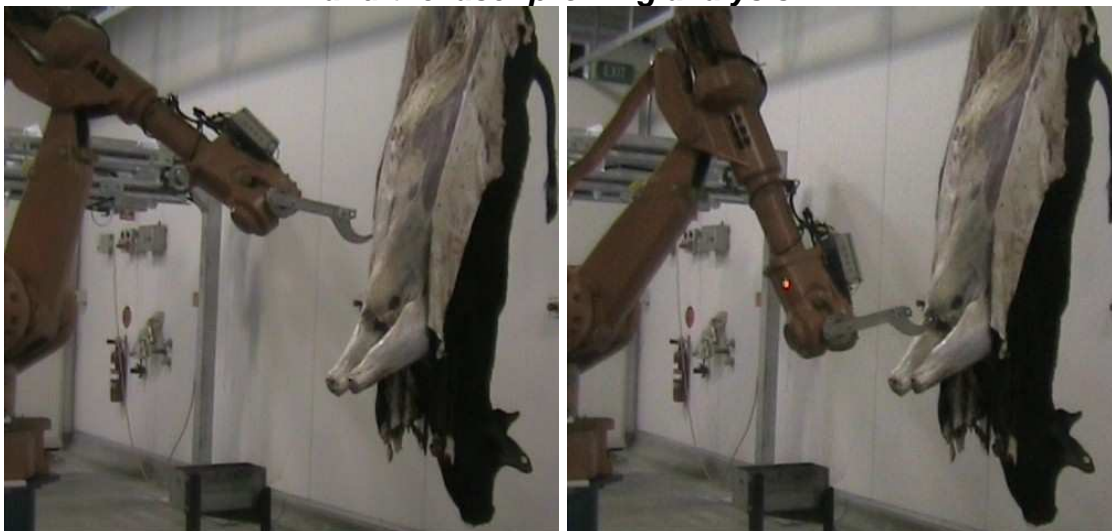
The sensing system is combined with the robot to demonstrate a fully automated brisket cutting system
