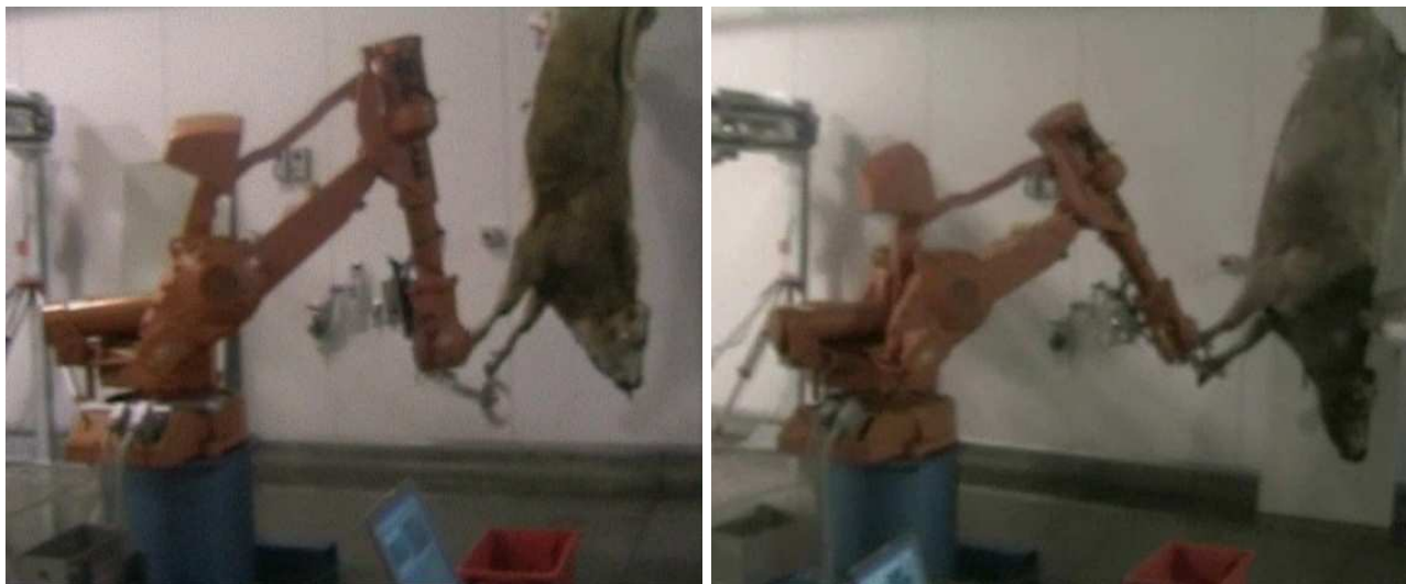
The sensing system is integrated to a robot to demonstrate a fully automated beef hock cutting system
