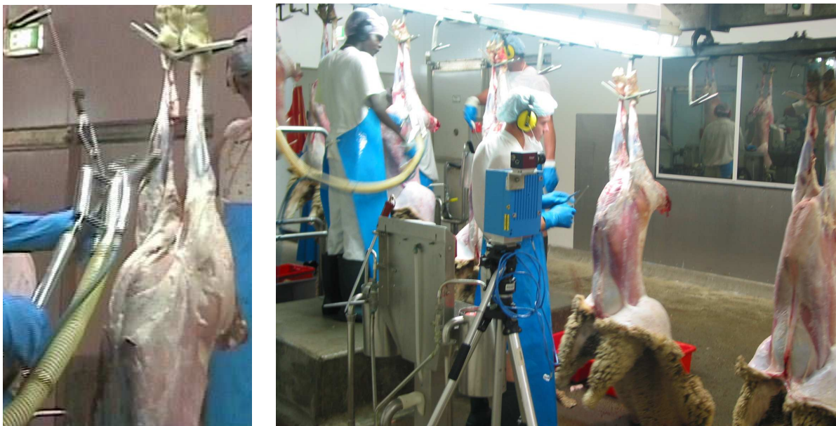
Manual Y-cut VacSan process and sensing system being demonstrated in a typical sheep plant
