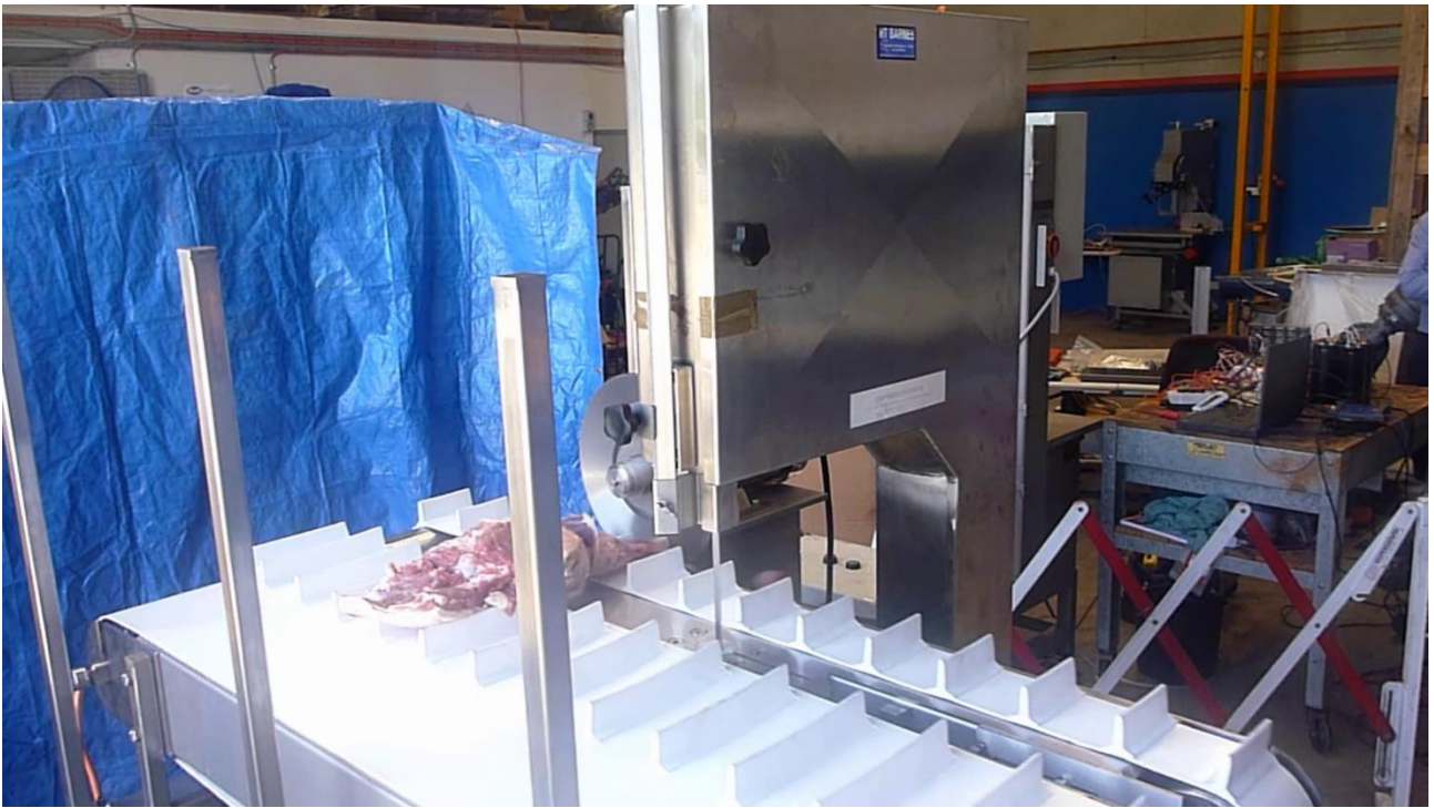
Figure 5: Product seen with both cuts completed, still on the conveyor and with tip ejection in progress
