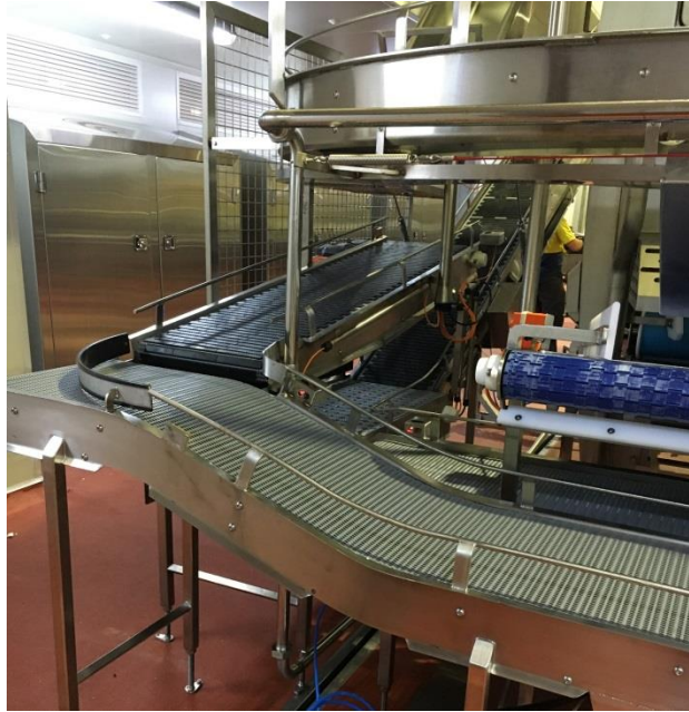
Figure 11: Multibatcher carton delivery system
