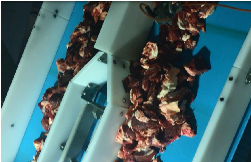
Figure 10: Trim distributed evenly across multibatcher feed belt
