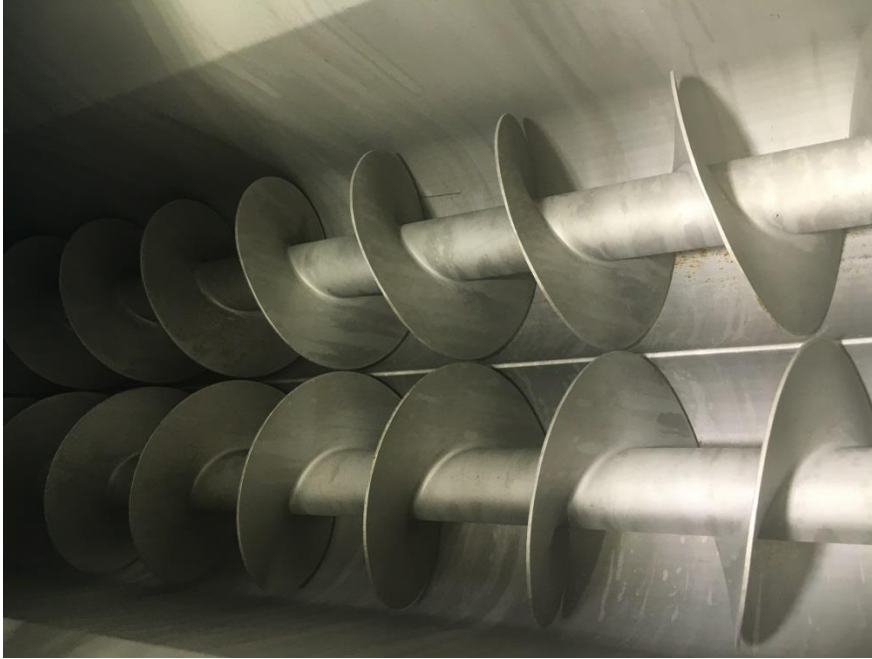
Figure 9: Counter-rotating twin screws
