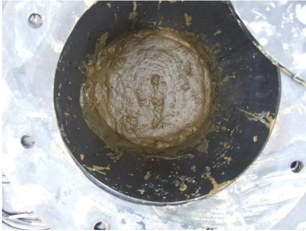
Photo 17: CAL crust at flare end
