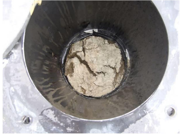
Photo 18: CAL crust at screen end
