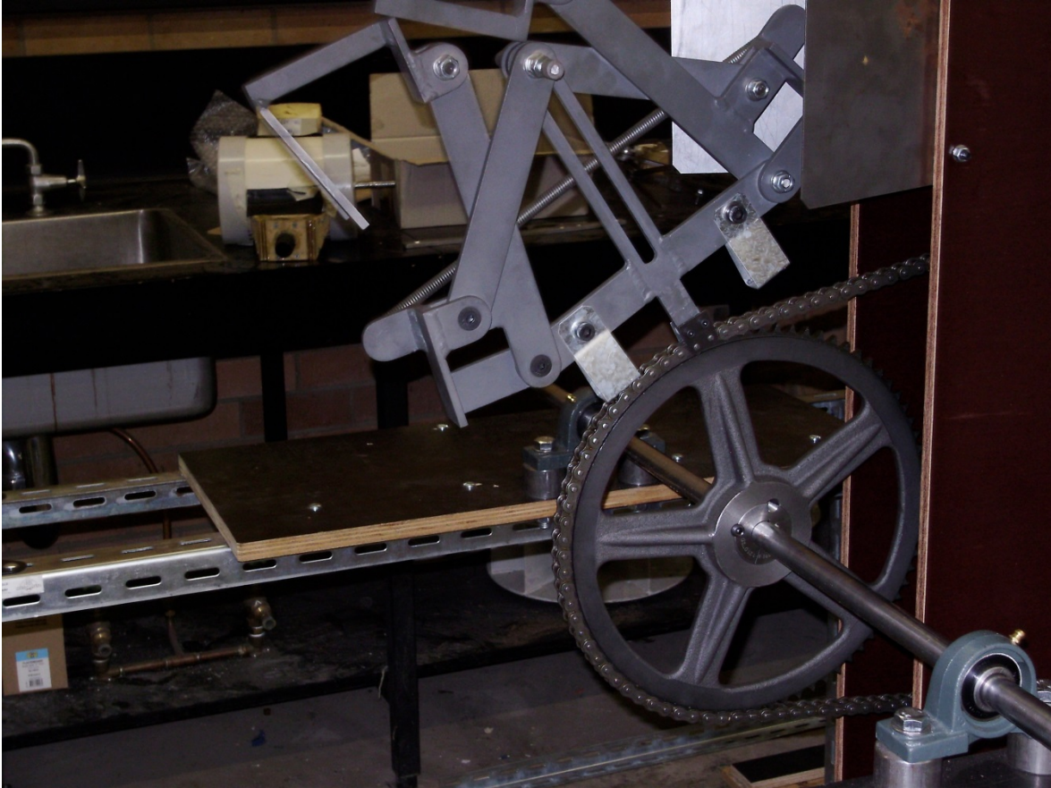
Figure 8: The second prototype integrated with the test rig and showing the shoulder supports that prevent it from rotating excessively relative to the chain under the influence of tripping and resetting loads.
