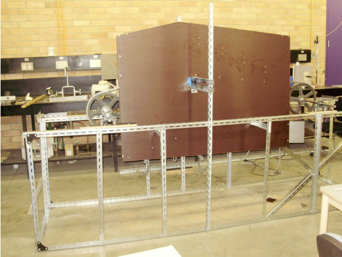
Figure 7: The final configuration of the test rig. The chain moves between the wooden constraining walls that also provide mounts for the tripping ramps. The positions of the tripping ramps are given by the double line of screws in the top right quarter of the wall, and the single line of screws in the bottom left corner.
