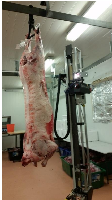
Fig. 19 - Scanning rig redesign employed in Lamb Carcass 3D and Hyperspectral data collection
