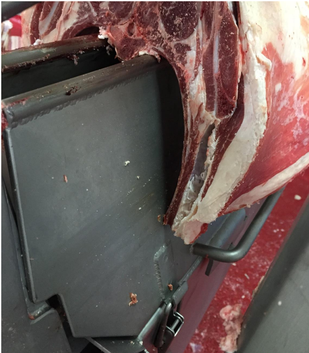
Figure 30: Gap at interface of loading station cover and product pusher chain cover is a snag point
