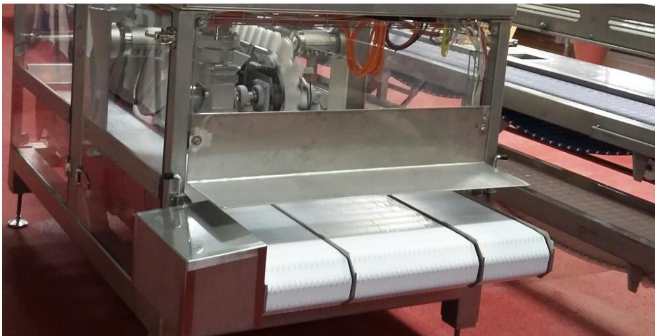
Figure 24: Additional guarding at end of product discharge conveyor
