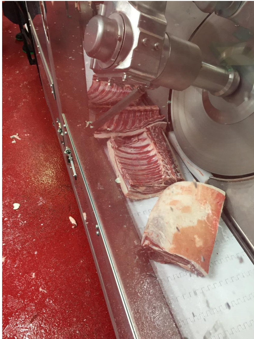
Figure 28: Large products are becoming stuck on the small conveyor
