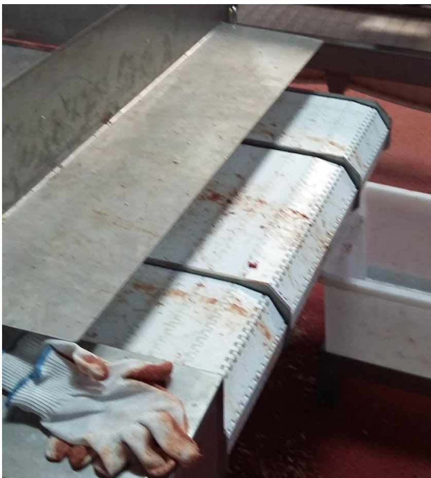
Figure 26: Product (Left and Right) and Bone (Middle) conveyors, all exit along the same line
