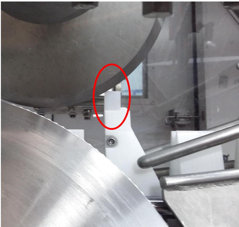
Figure 17: Replaceable product pusher inserts come into close proximity of cutting blades
