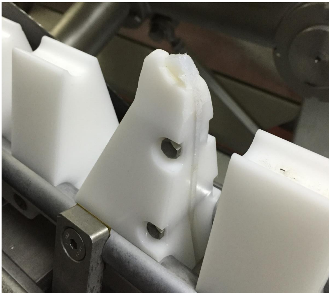
Figure 31: Worn down product pusher and wear insert
