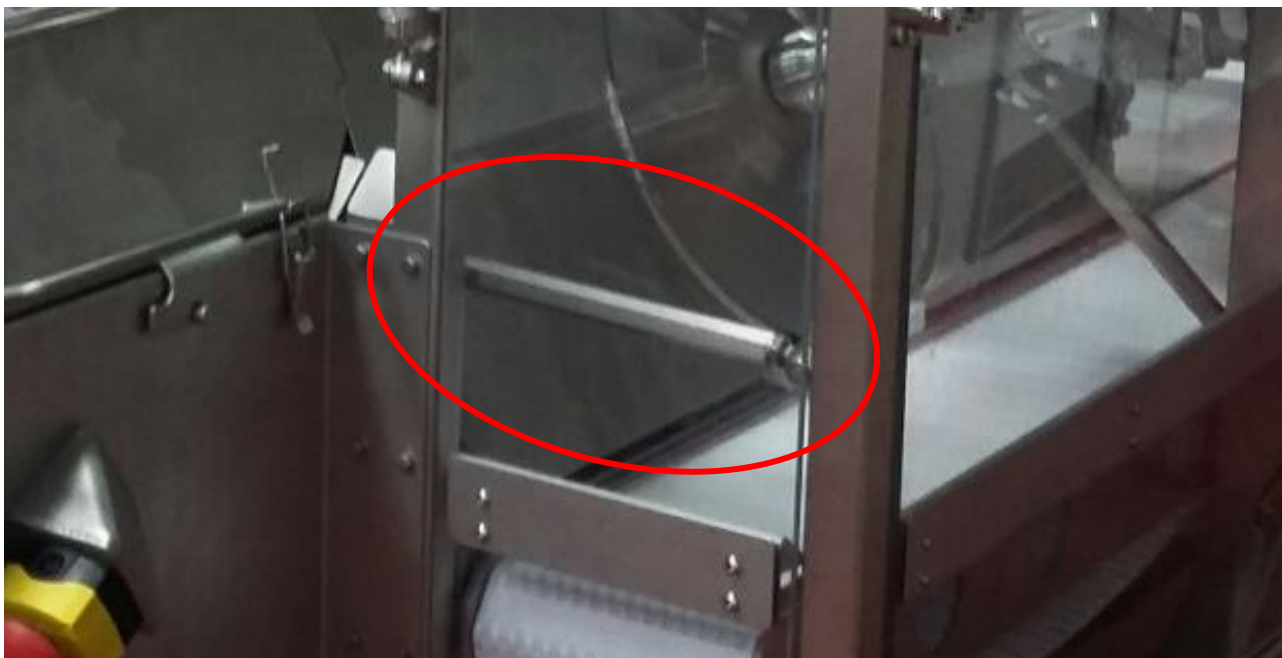
Figure 25: Rod eye that controls the horizontal position of the product chain - Needs revision
