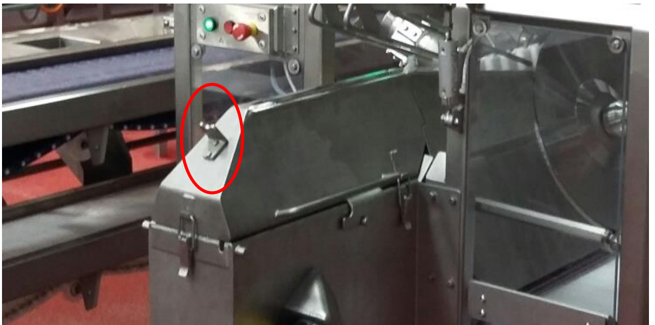
Figure 20: Spine scraper installed onto loading station
