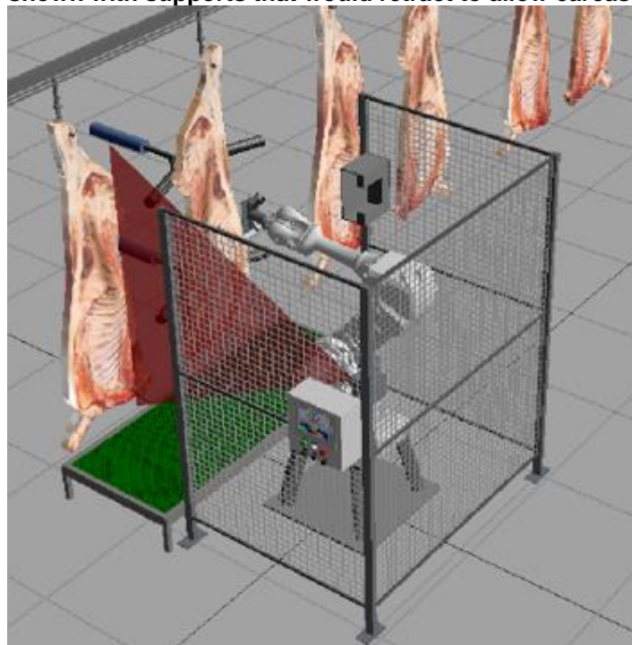
Fig.24 Indexed system, shown with supports that would retract to allow carcasses to index.
