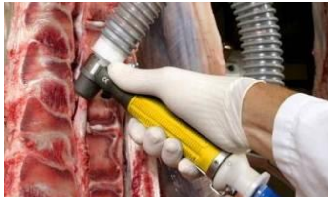
Fig. 7 Bettcher Industries Vacuum tool with internal cutter
