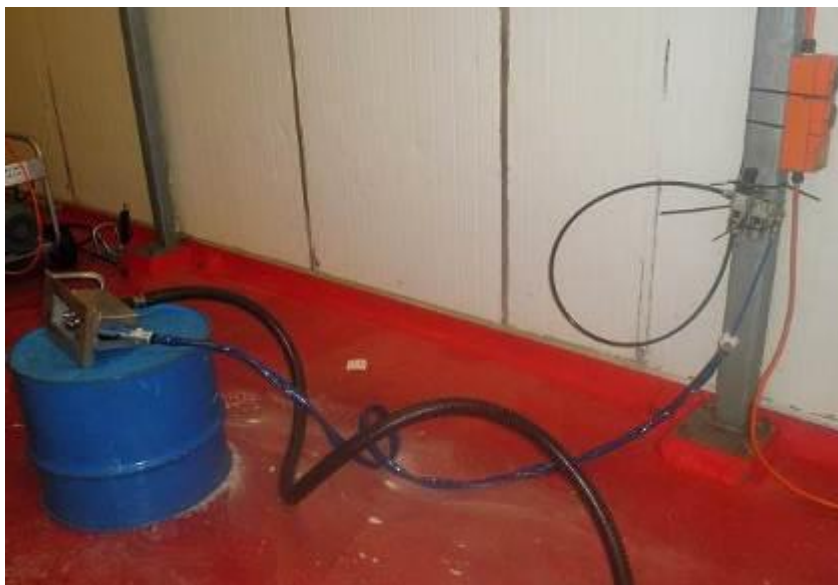
Fig.16 Equipment setup for converted manual cutting tool, the connection to the air supply and vacuum unit are shown.
