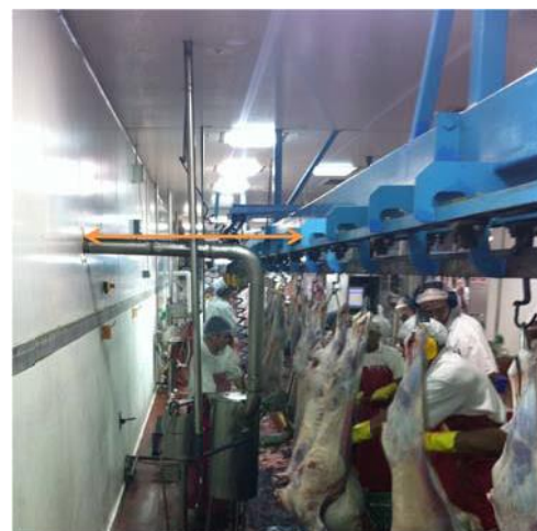
Figure 18: Distance between wall and slaughter chain for manual or MAR brisket cutting may require recessing into wall
