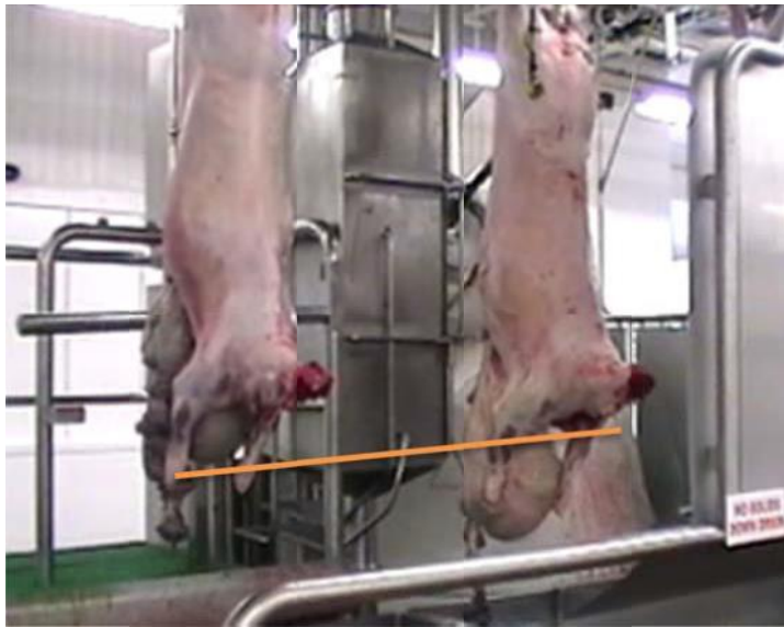
Figure 3: Auto Evisceration accommodates carcass weight ranges
