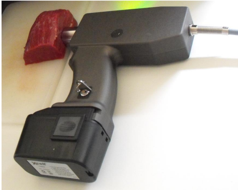
Figure 2. Measuring the SM with a Raman hand held probe, perpendicular to the muscle fibres.
