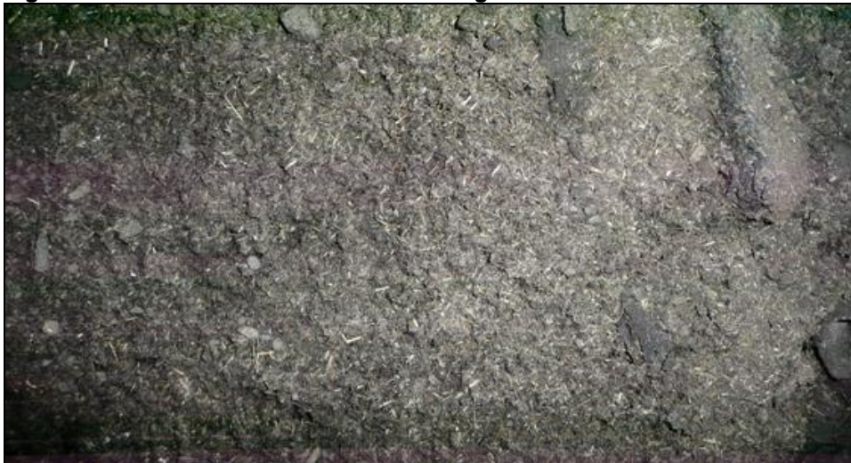
Figure 4.3: Picture of dewatered DAF sludge
