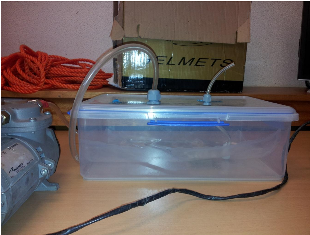
Figure 3.5: Evacuated container method for collecting biogas. The tube on the left is connected to the pump which draws a vacuum on the container. A tube connected to the cover would be connected to the tube on the right, which is attached to a Tedlar bag inside the container. The vacuum drawn by the pump forces the Tedlar bag to draw gas into the bag for collection.
