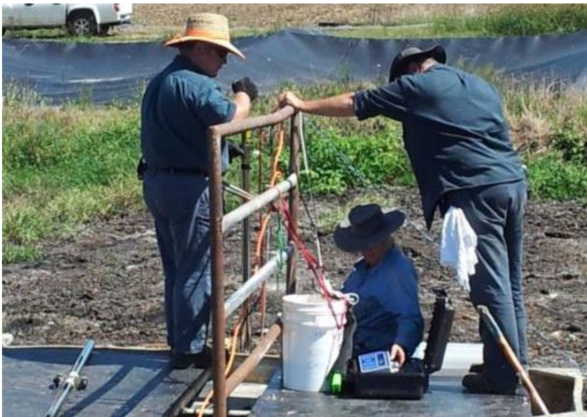
Figure 3.7: Monitoring water conductivity, pH and sampling the sludge from the base of pond A. The depth of the pond was 4.3 m. The white bucket later modified to clear fat and grease from the surface water, is tied to the frame.
