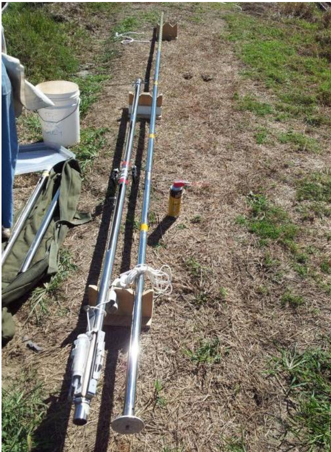
Figure 3.6: Prototype sludge depth pole (right hand side) and the monitoring and sludge sampling sleeve (left hand side).
