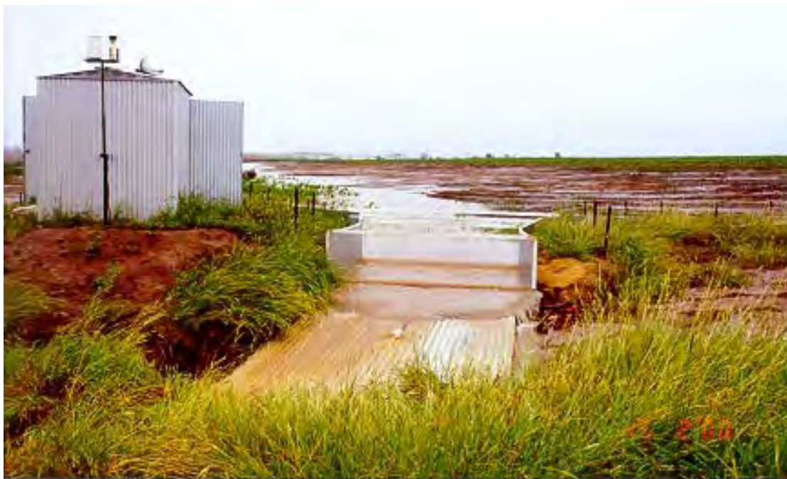
Figure 3: Paddock-scale equipment monitoring runoff (Feb 2000) in CP trial
