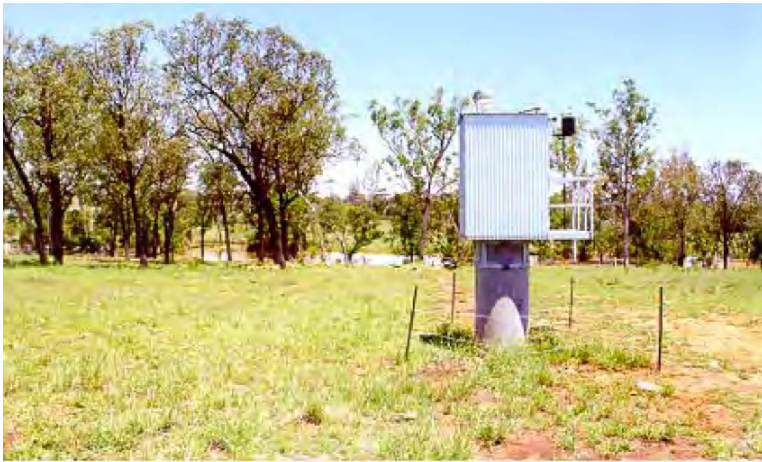
Figure 7: Catchment scale electronic equipment measuring stream depth, rainfall and water quality.
