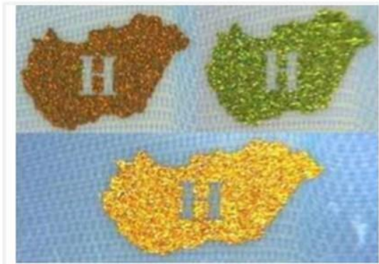
M 1 * * * OVI (Optically Variable Inks) (For. Showing a large colour shift for validation)
