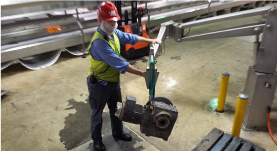
Figure 3. Commercial lifting trials at JBS Brooklyn using mobile hydraulic lifter as manual assist in the workshop environment.
