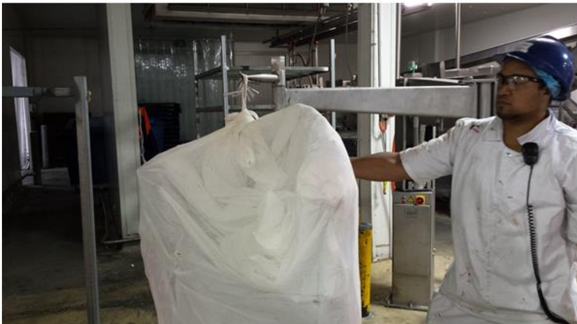
Figure 4. Commercial lifting trials at JBS Brooklyn using mobile hydraulic lifter to demonstrate safe lifting of beef quarter beef.
