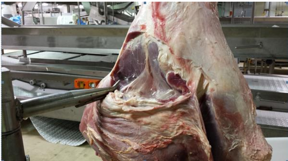
Figure 7. Commercial trials at JBS Brooklyn using mobile hydraulic lifter to demonstrate boning assistance on beef butts.
