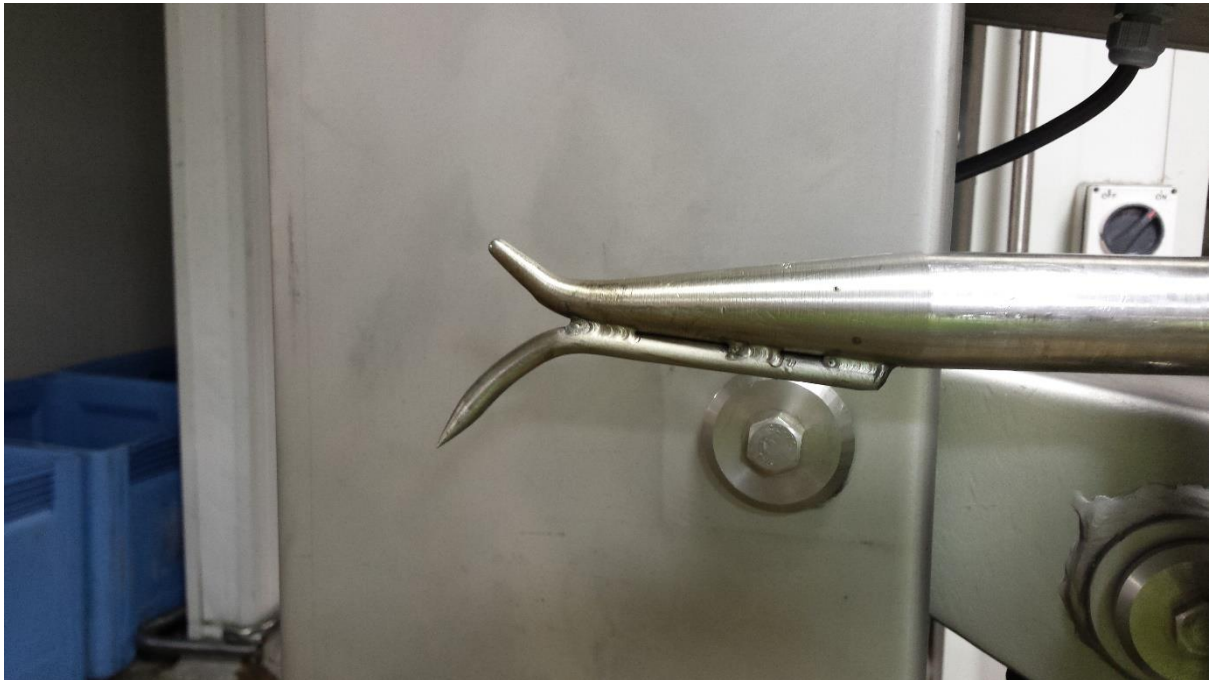
Figure 11. Commercial unit with modified end effector to allow pulling applications
