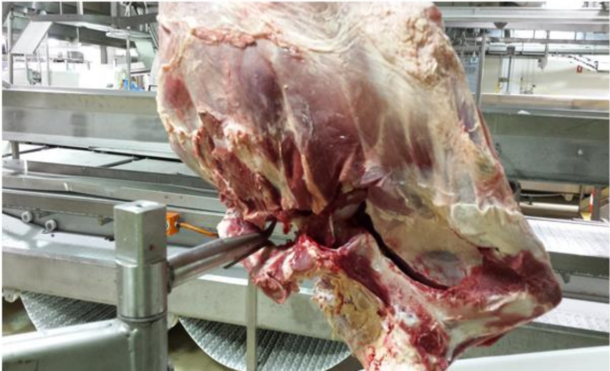
Figure 6. Commercial trials at JBS Brooklyn using mobile hydraulic lifter to demonstrate aitch bone pulling on beef.
