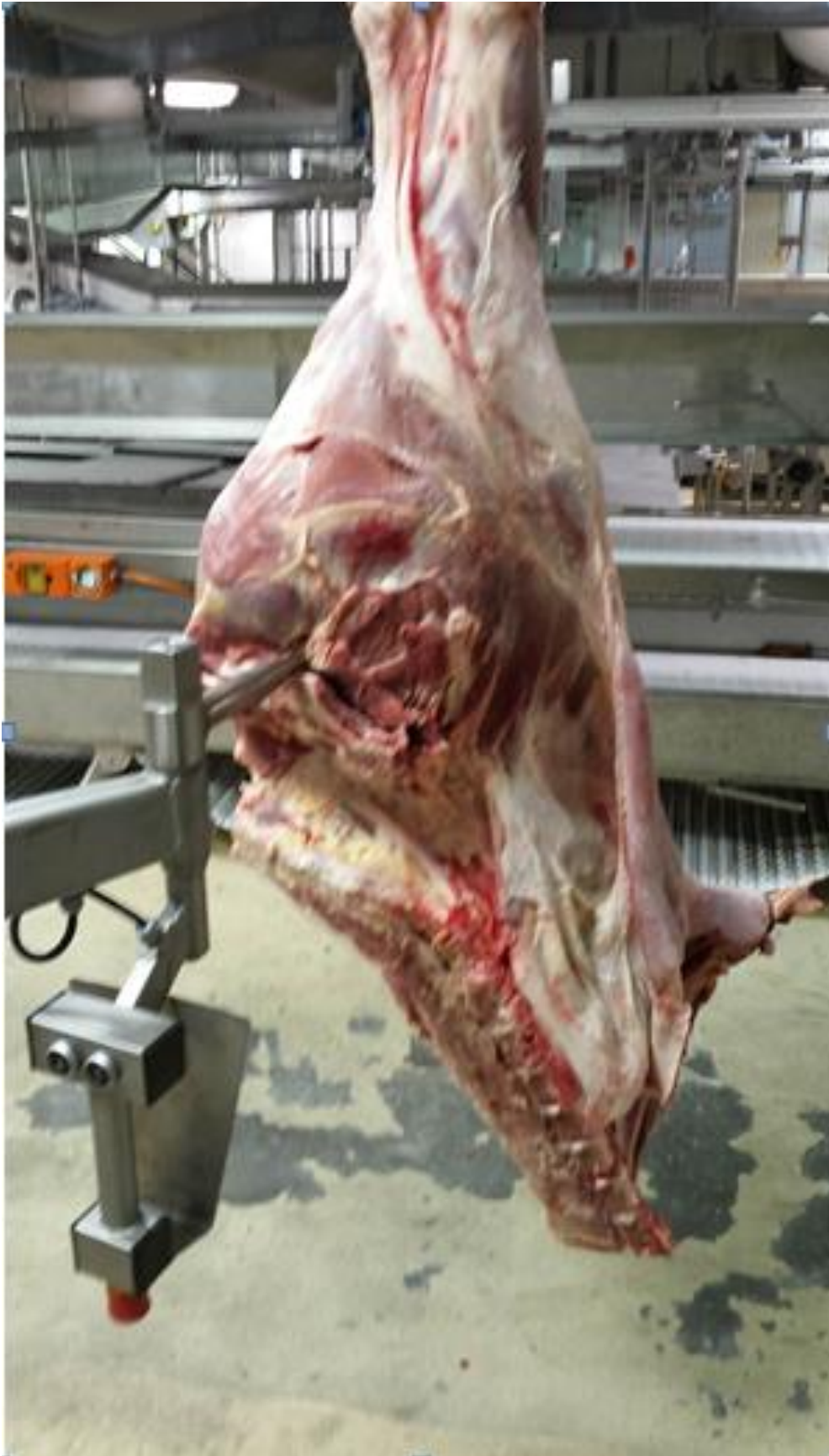
Figure 5. Commercial trials at JBS Brooklyn using mobile hydraulic lifter to demonstrate aitch bone pulling on beef.
