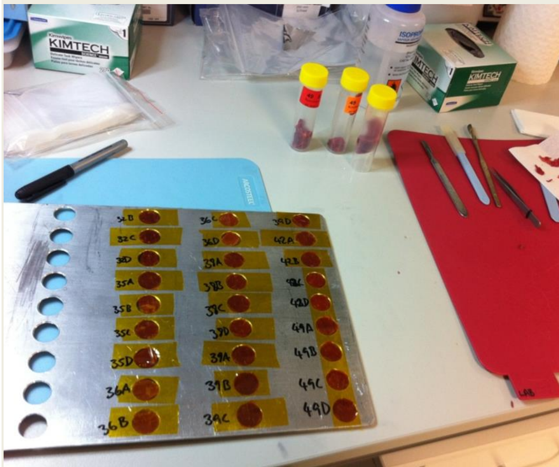
Fig. 4. Four subsamples cut into 2 mm thin slices and fixed to the sample plate using tape for the SAXS testing.
