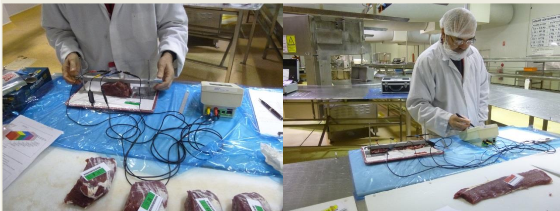
Fig. 3. Bioimpedance measurement of topside (SM – picture left) and loin (LL- picture right) muscle samples post mortem
