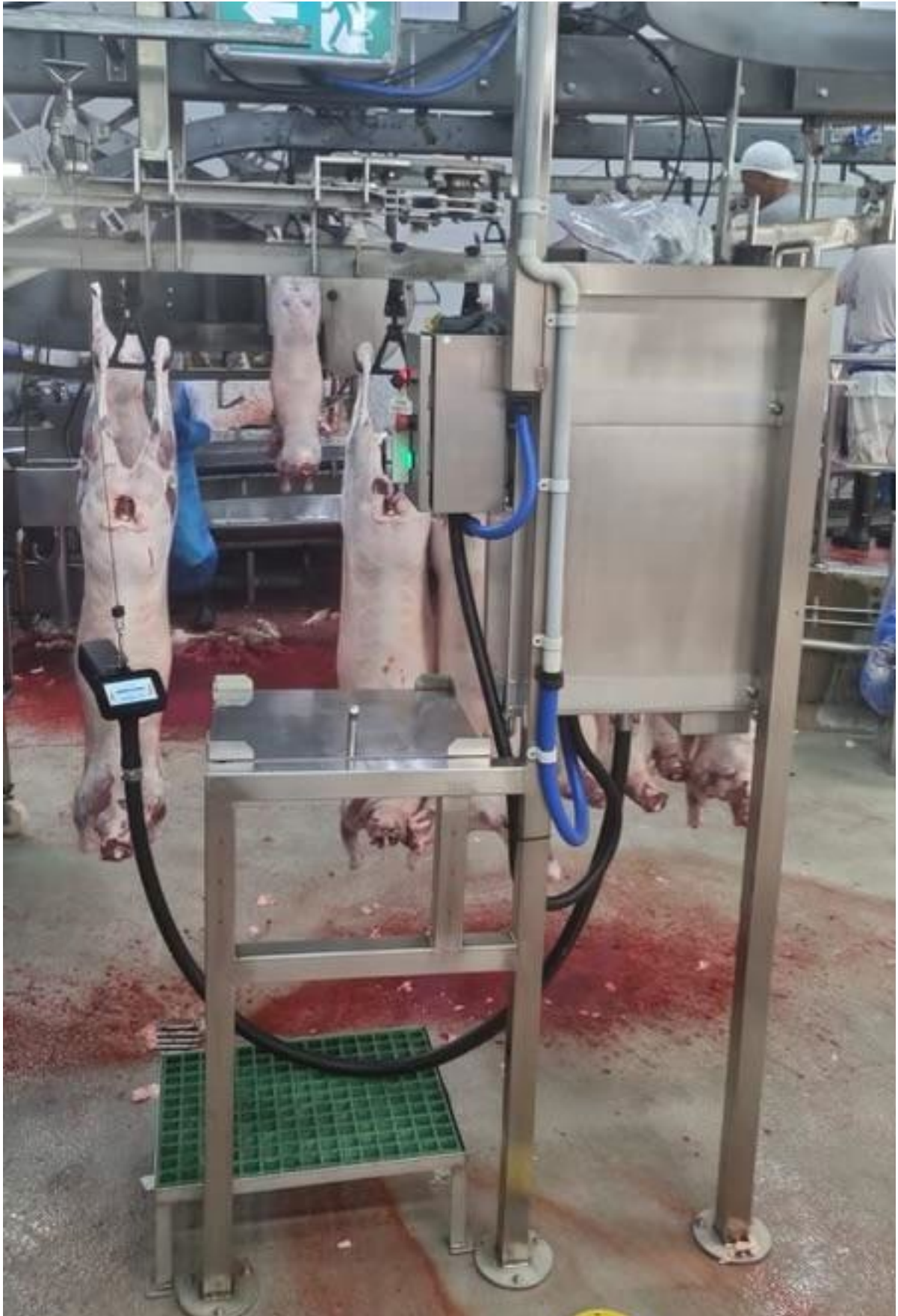
Photo 3. MEQ Probe fully installed at Frews.
