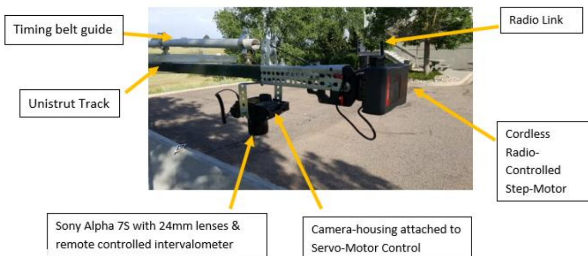
Figure 2: Image of the experimental motorized trolley with camera
