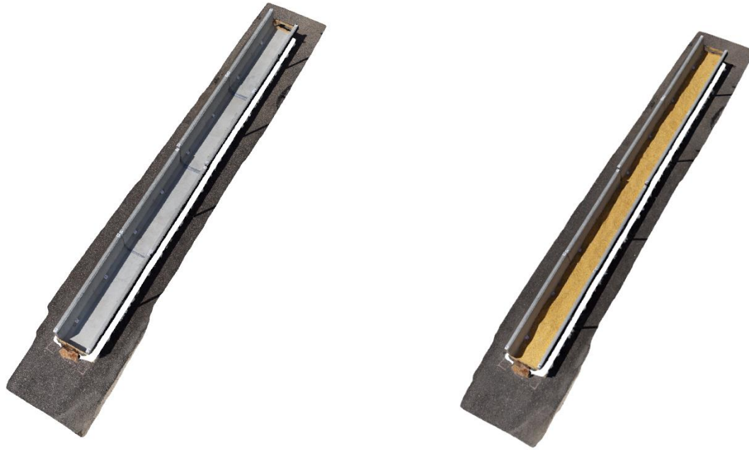
Figure 5: Empty and full troughs modelled based on multiple images taken by the constructed system
