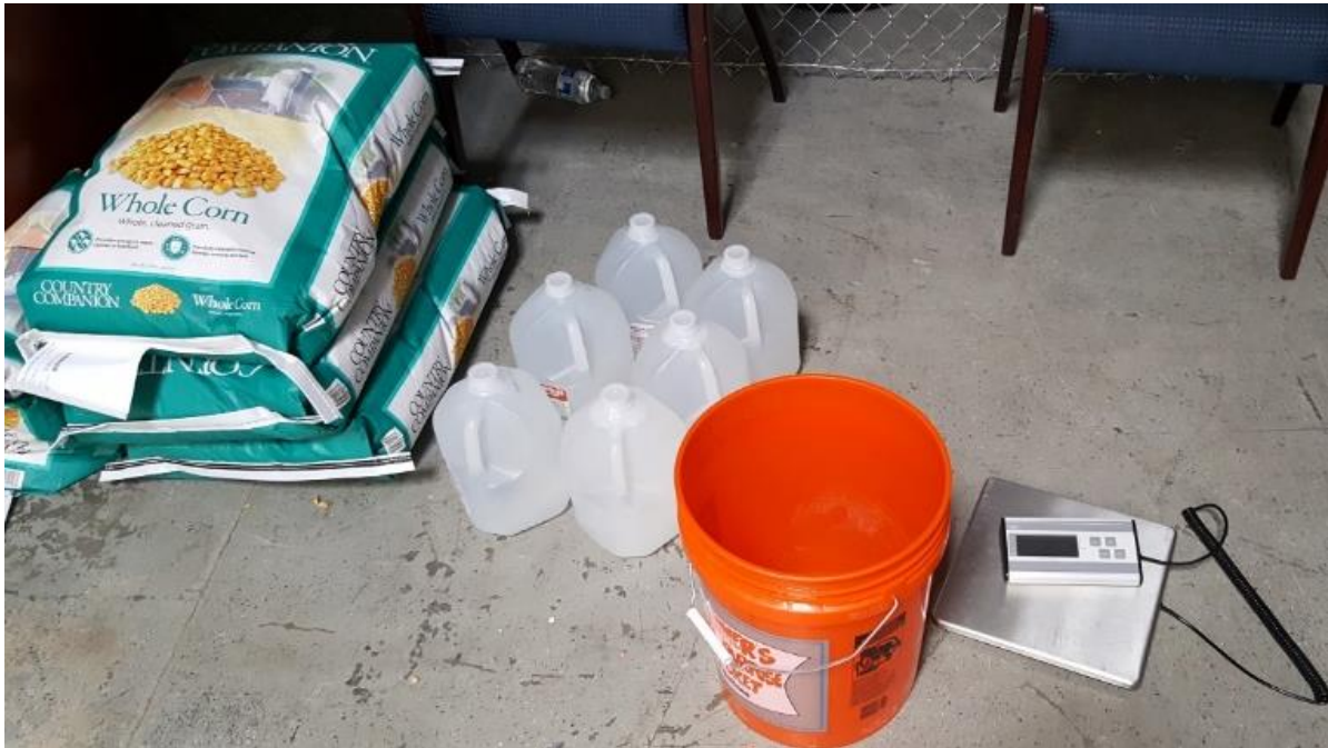
Figure 10: Confirming the specific weight of the used corn with a comparison to distilled water
