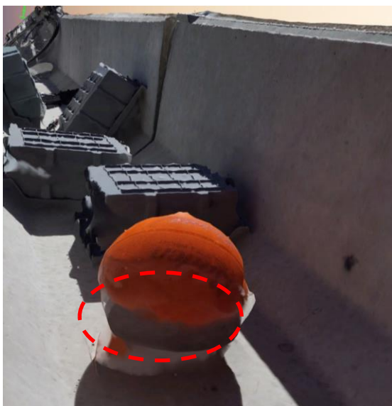
Figure 8: A basketball photogrammetrically modelled. You can see artefacts of the computer modelling.
