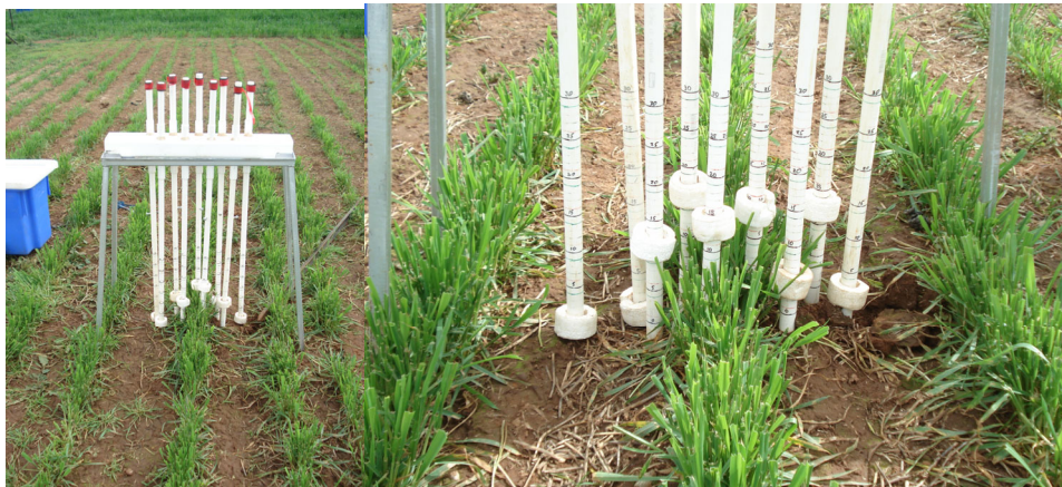
Fig. 3.4. Device used for measuring changes in height across wheat swards.
