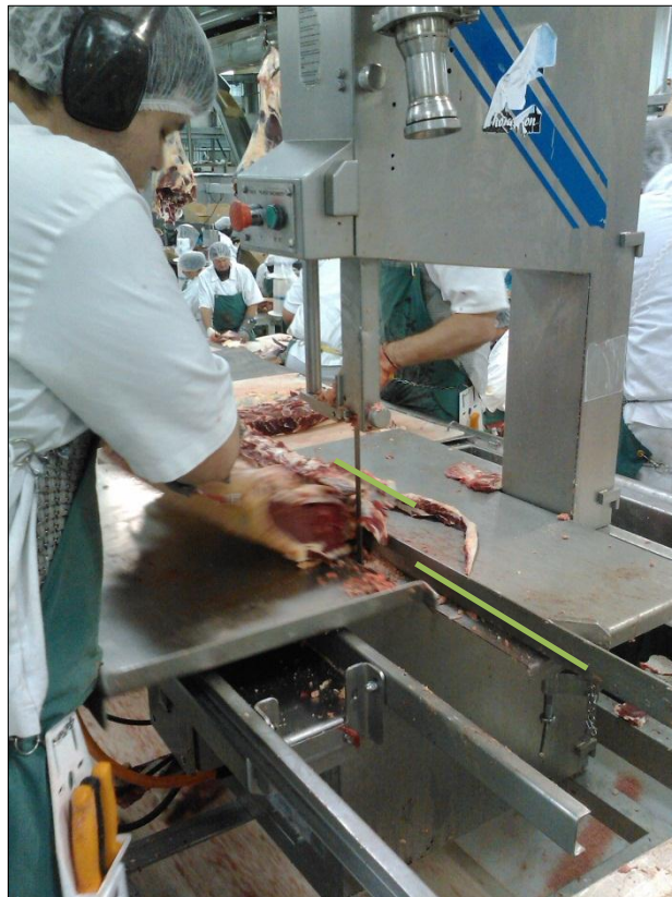
Figure 14 - Side operation of a band saw (Source: Taken by Tim Phillips during project orientation 7.10.11) Note: Green laser line superimposed
