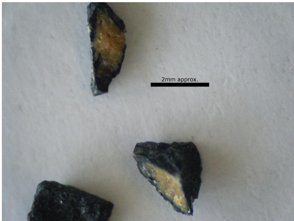
Figure 15: Iron sulphide deposition on media obtained from the Zetos filters.
