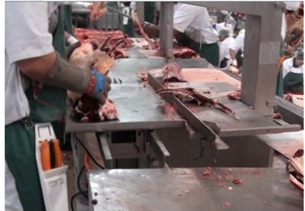
Sliding Table Bandsaws – adaptable to meat holding jigs
