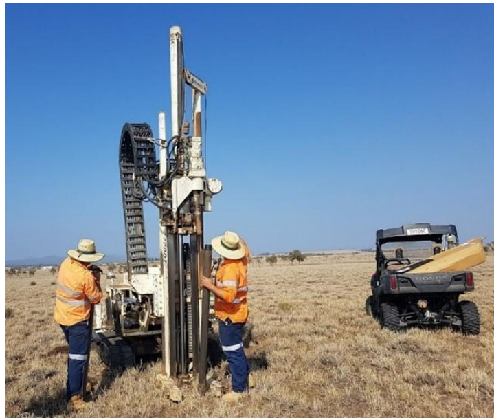
Figure 2 - Extracting soil cores with a hydraulic coring rig
