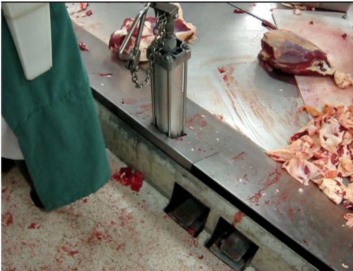
Figure 1: Modified and immobilised pedal operated JBS knuckle puller station.
