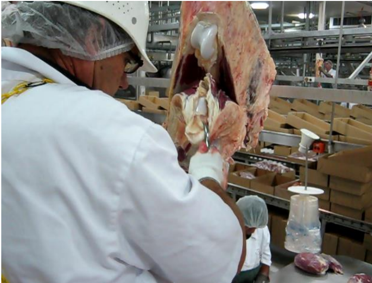
Figure 3: Removal of beef knuckle assisted by the modified JBS puller.
