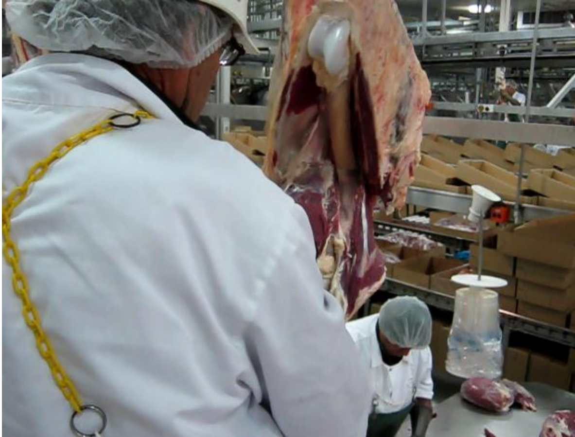
Figure 4: Clean bone removal of beef knuckle using the modified JBS puller.
