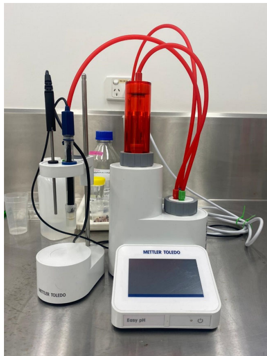
Figure 13: The Mettler Toledo Easy bench-top pH meter used as the Golden standard.
