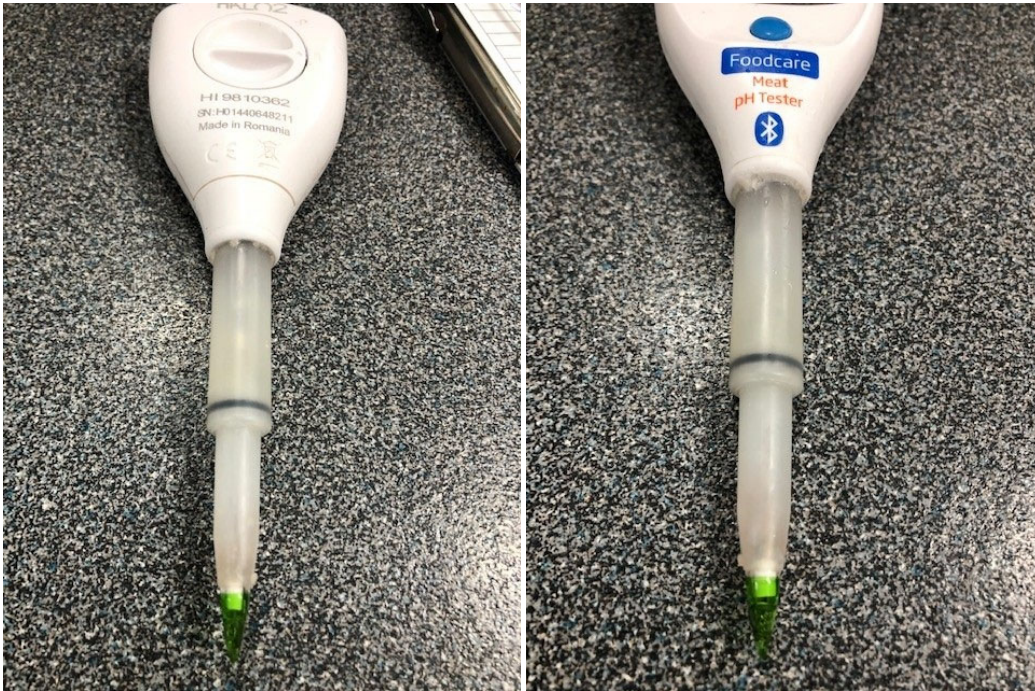
Figure 38. The HALO2 probe after 20 readings showing fat/meat juices under the sleeve.
