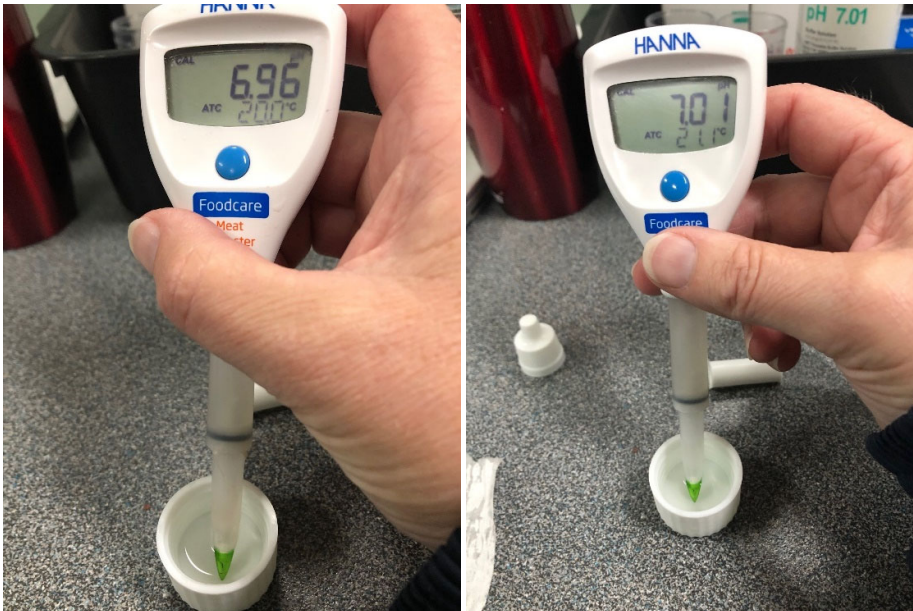
Figure 39. The HALO2 probe indicating the impact of the aperture being 'dirty' (left image) versus 'clean' (right image) when placed into the pH 7.01 buffer solution.
