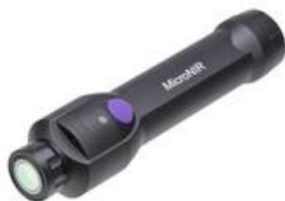
Figure 7: A typical small hand-held Micro-NIR meter suitable for on-line carcass scans.
