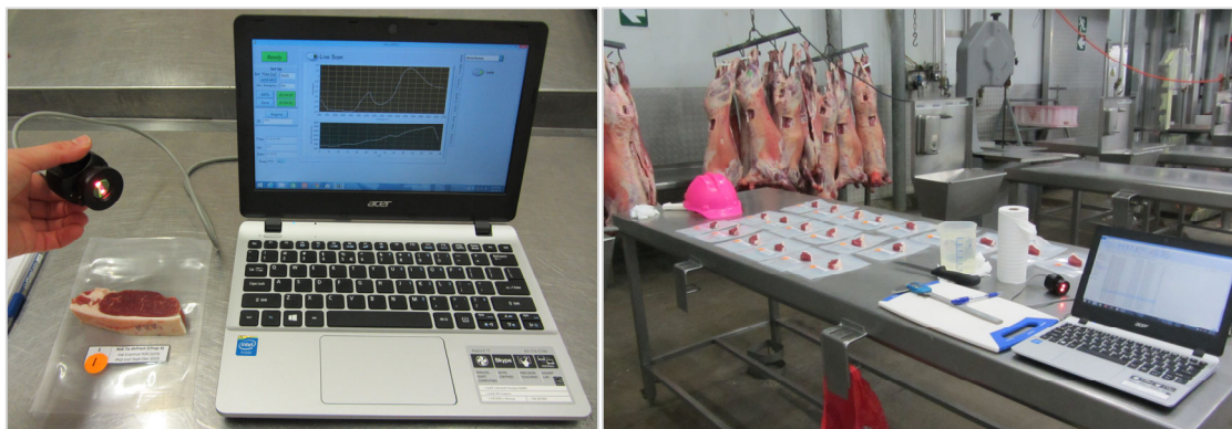
Figure 8: Practical measurement set-up for a lamb meat steak quality measurement using a Micro-NIR (45 mm in diameter and 42 mm in height, weighing 60 g).
