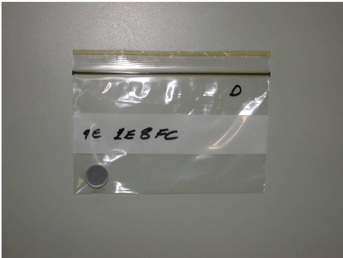
Figure 2: iButton logger used to record meat surface temperatures
