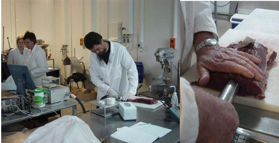
Figure 1. Meat being measured with KES NIR spectrophotometer.
