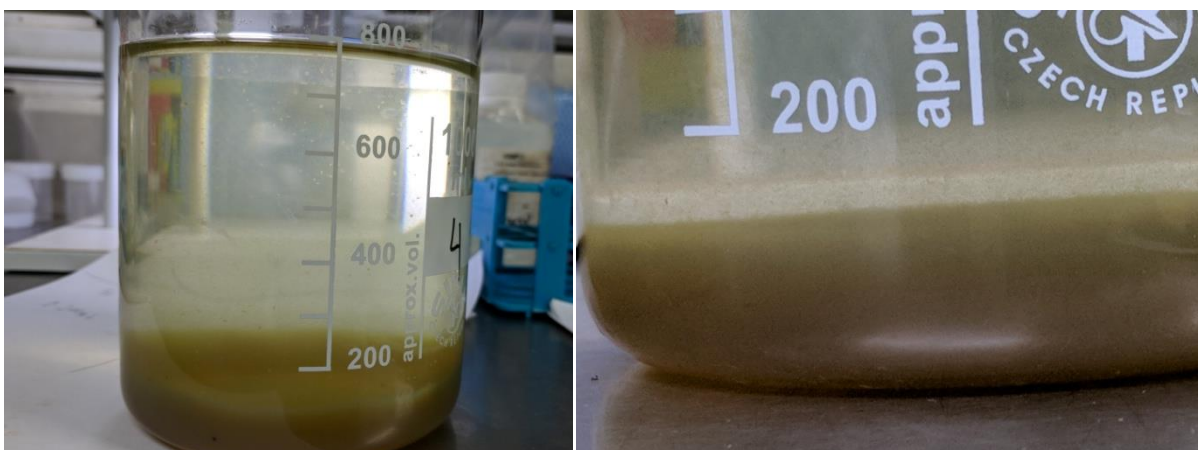
Figure 3. Settled sludge produced during dosing trials
