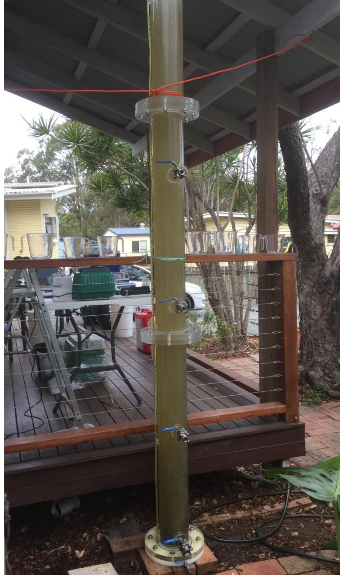
Figure 4. Settling column full of lanthanum chloride dosed effluent, prior to settling
