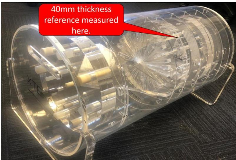
Figure 3. A simple thickness measurement was taken within the XTE-CT test piece using the section shown which was designed to be a uniform 40mm thickness.
