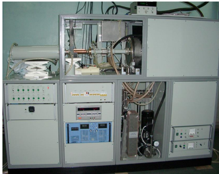
Figure 1. Side view of the 28GHz, 15kW Gyrotron at IFP without modifications
