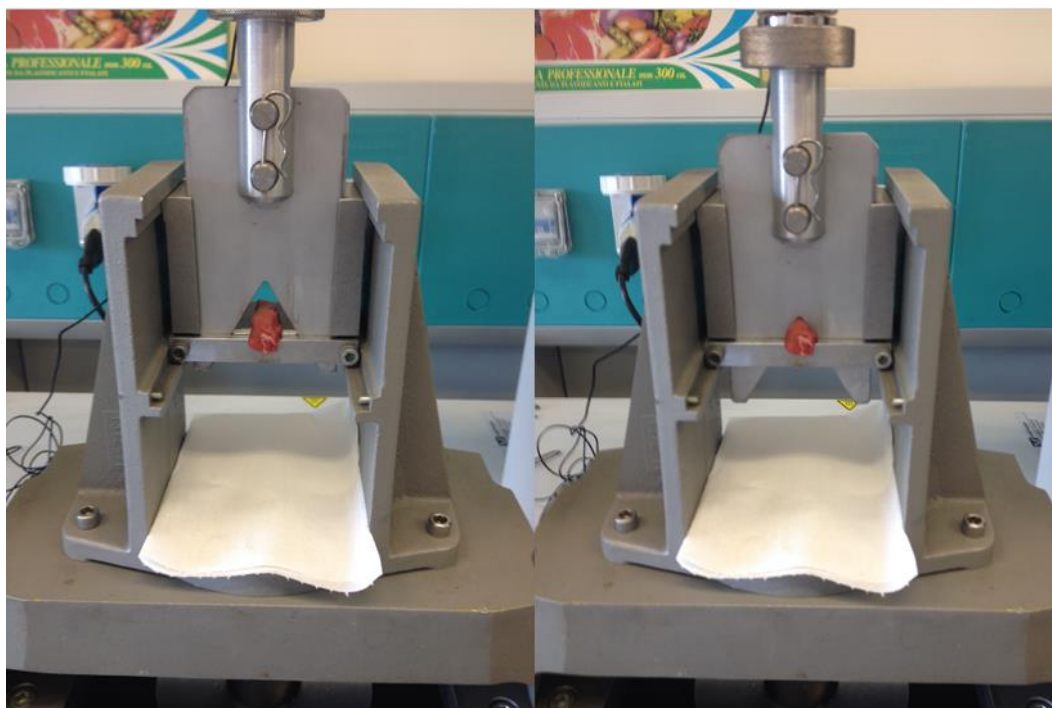
Figure 3. 3365 Instron Universal Testing Machine with a shear-cutting blade (Warner Bratzler blade) to identify shear force value at DeFENS
