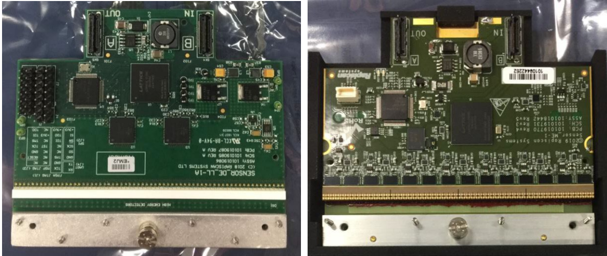
Side-by-side comparison of dual-energy (left) and multi-energy (right) detector boards. The line of x-ray detection is horizontal across the lower part of the board.
