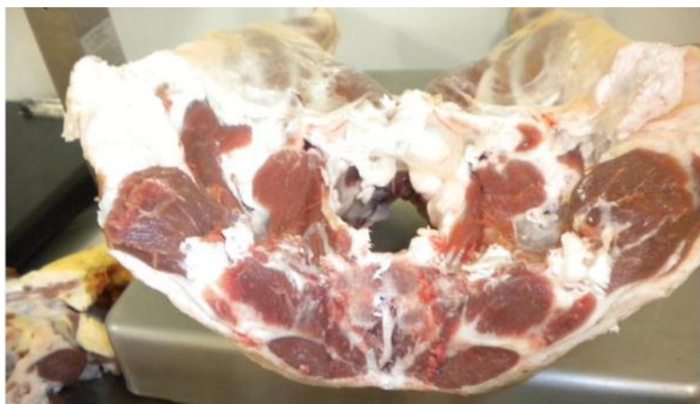
Figure 34: Lamb hindquarter cut with the LEAP III x-ray primal cutting system, note cut meat surface and lack of bone dust present.
