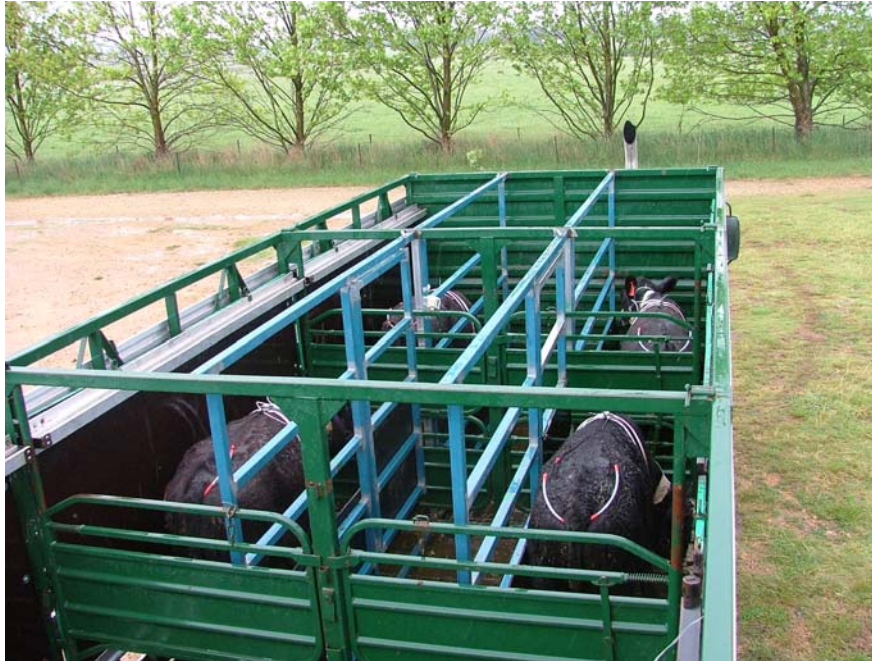
Figure 1 Modifications to stock crate and cattle position during transport
