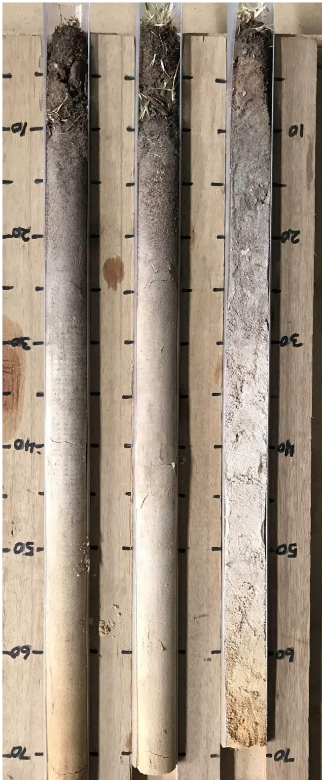
Figure 8: Cross-section of 'Mid slope' soil test site
