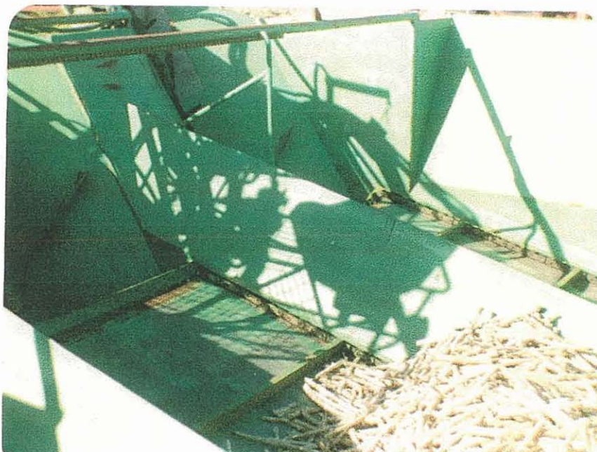
F.9 Three-row Moller planter; each of three bins had a moving slat floor to pull the cuttings towards the front shutters; operator on the planter had control over rate of movement of each floor
