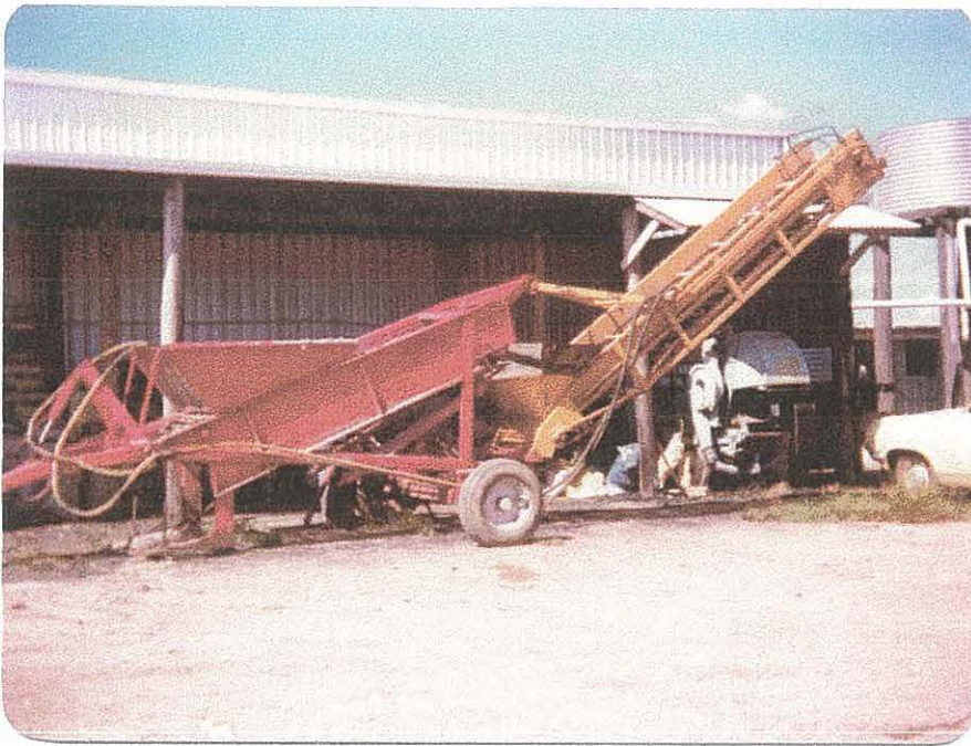
F.1 Early version of cassava root harvester; important feature is concave cutter bar and debris splitting posts
