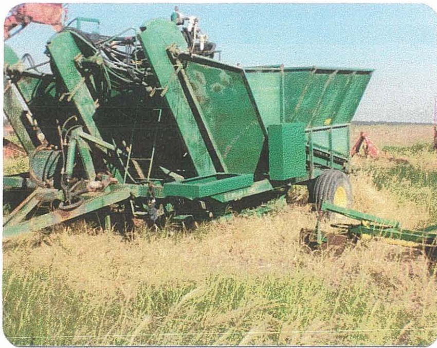
F.7 Three-row Moller planter; planted billets in 1.5 m rows at 13,000 to 18,000 per ha
