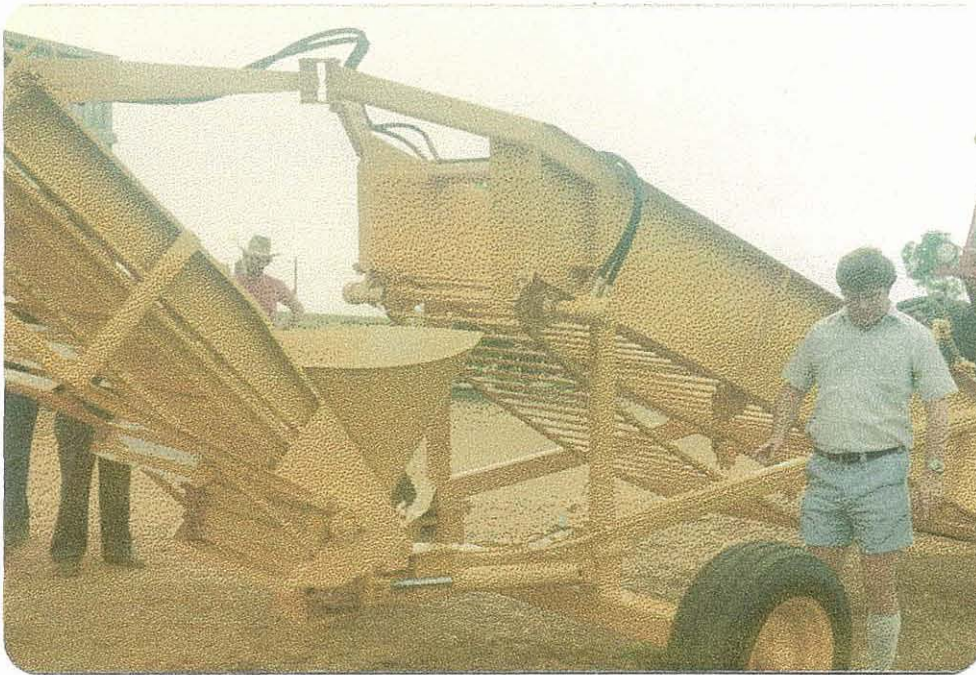
F.2 Cassava root harvester; Toft prototype May '80; the front elevator/cleaning shaking bar remained part of the final harvester as did the rear loading elevator
