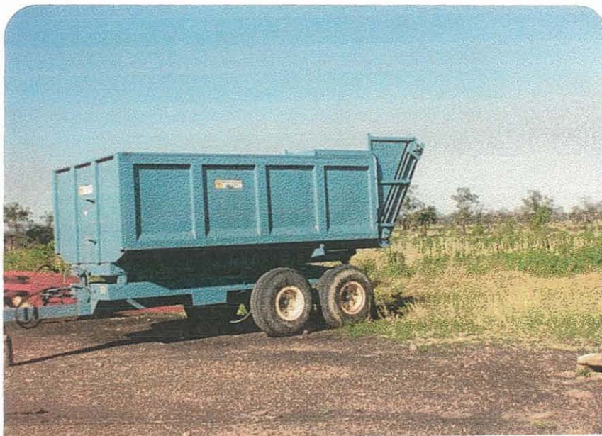
F.6 Haul-out bin fitted with slotted elevator to regulate out-feed.
