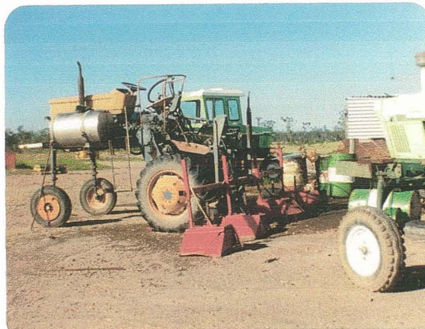
F.15 Shielded boom sprayer for delivery of herbicides and very high clearance tractor
