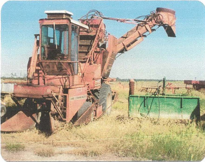
F.4 Cutting Harvester; a modified MF201 cane harvester with front crop gatherers removed and replaced with counter-balance front weight; used to harvest tops and prepare billets for planting
