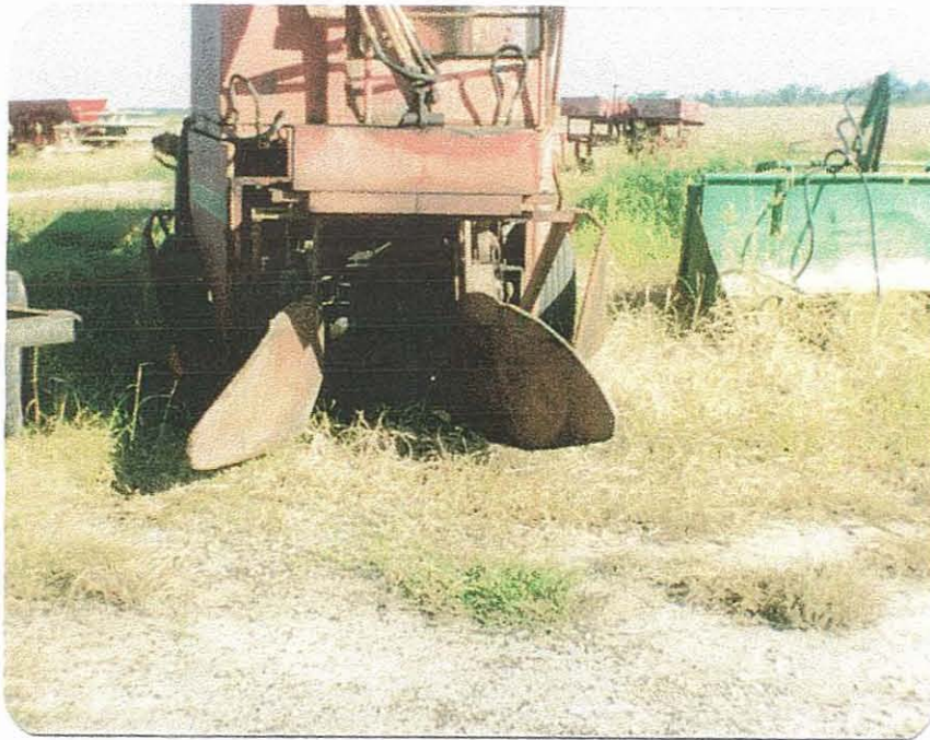
F.5 Cassava cutting harvester; front end modification which smoothed the flow of stems into the machine throat.
