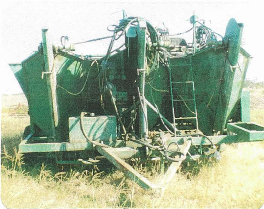
F.8 Three-row Moller planter; trailed by a 70-75dbKW tractor; one operator attended the planter
