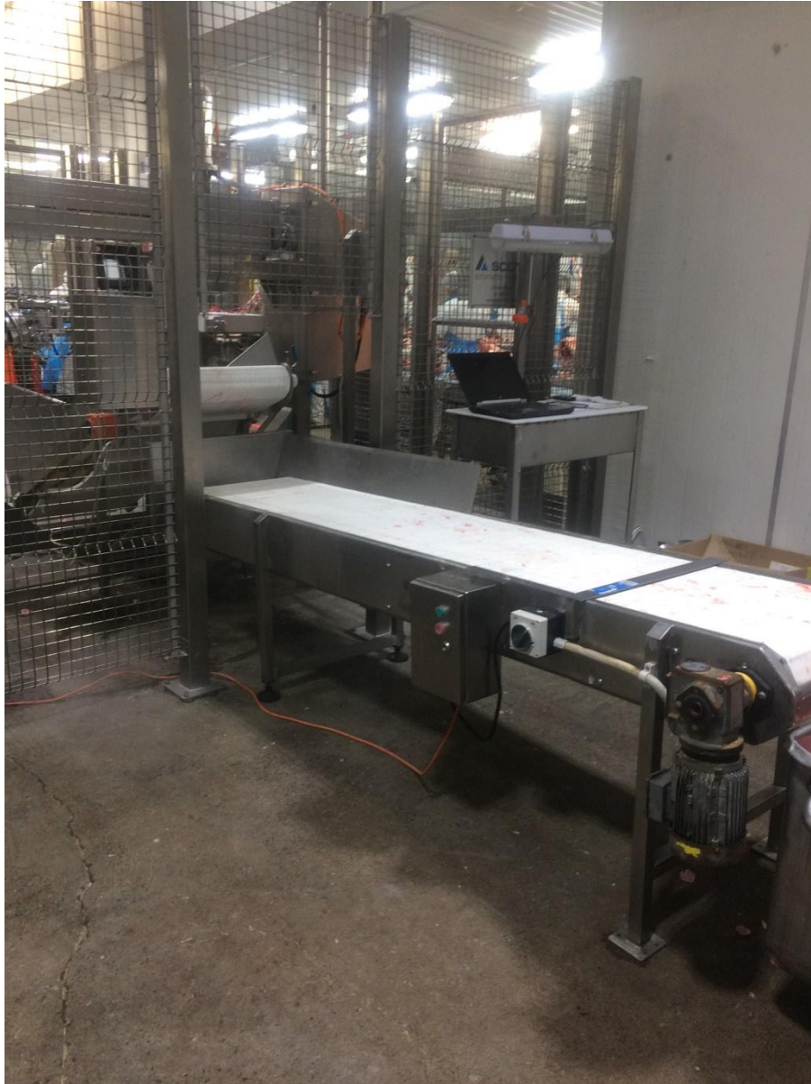
Fig. 50: Placeholder Outfeed Conveyor
