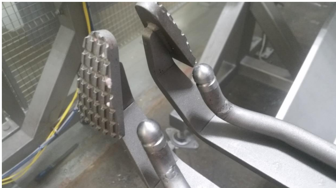
Fig. 16: Modified Locating Pins
