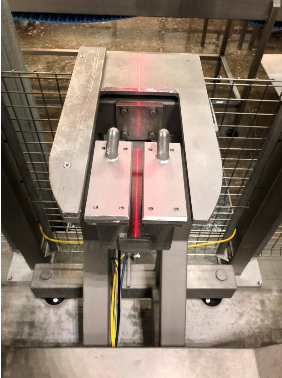
Fig. 23: Load Table with Alignment Laser
