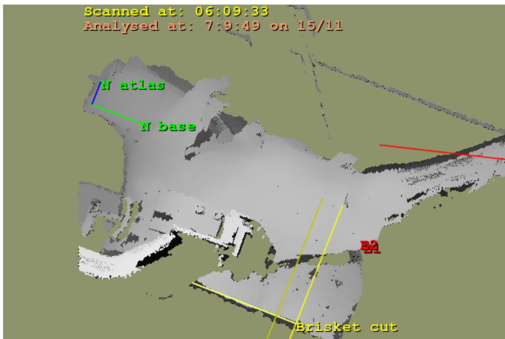
Fig. 52: Vision Scan with Light Interference
