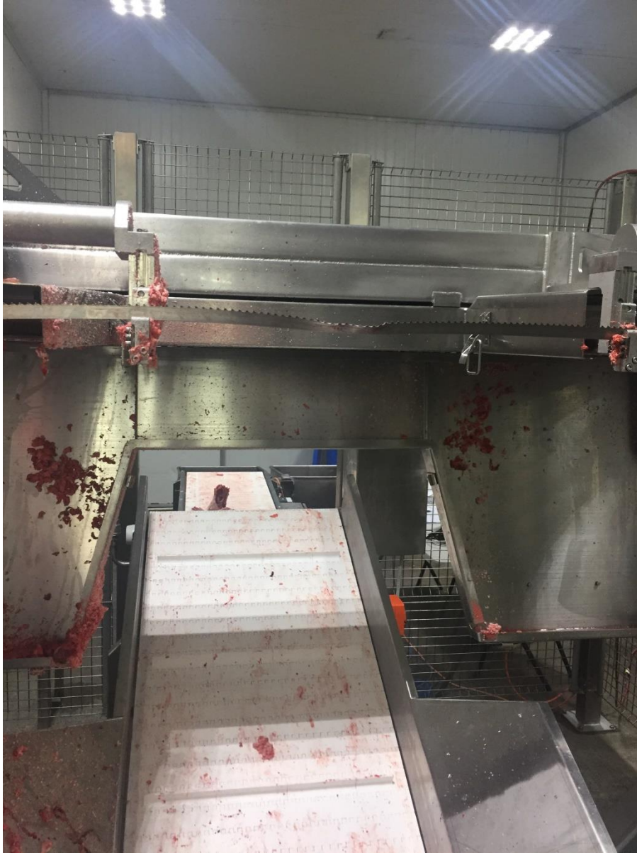
Fig. 21: Adjusted Left Bandsaw Blade Guide to Fix the Issue of Excessive Blade Deflection and Damage as in the Image Above. The issue has been fixed by modification of guide, bearing, and shaft.
