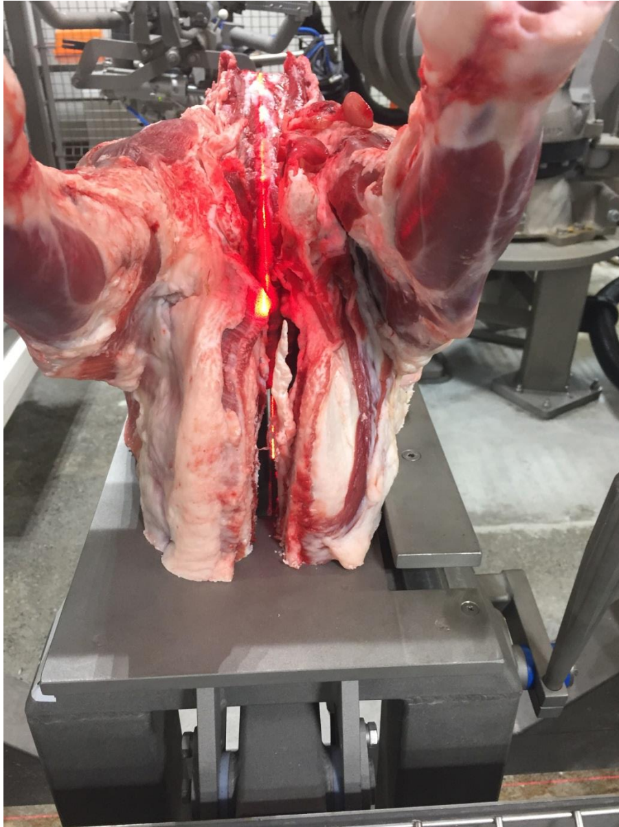
Fig. 40: Product on Load Table following Alignment
