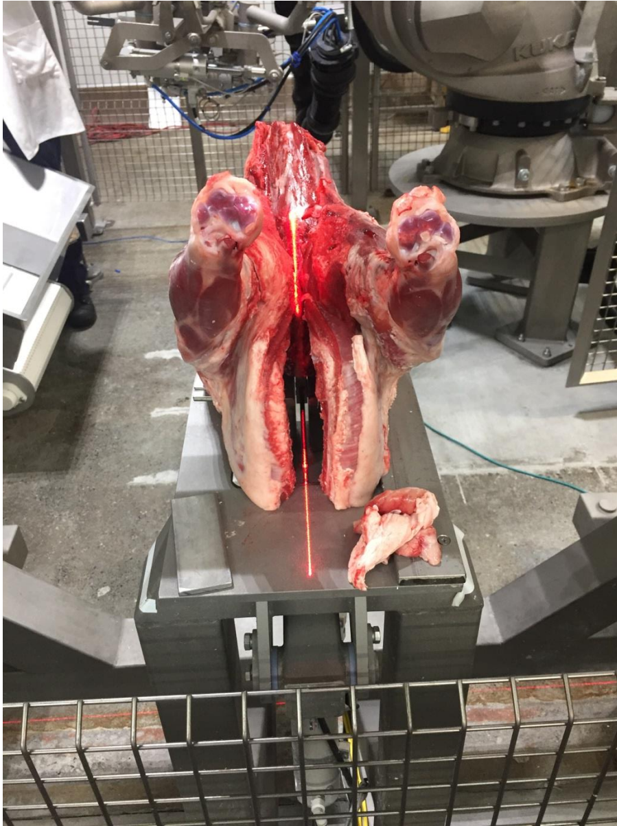
Fig. 24: Alignment Laser Projected on Product
