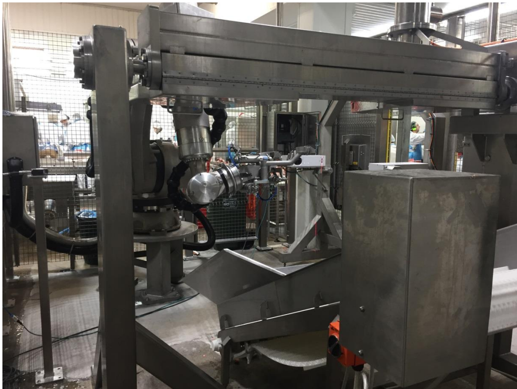
Fig. 11: Robot with Gripper, Bandsaw, and Product Conveyor 2
