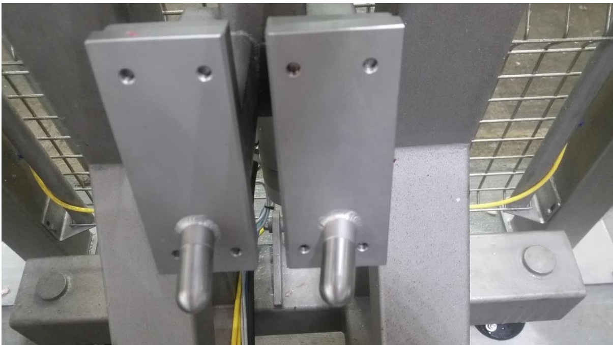
Fig. 13: Modified Load Table Locating Pins
