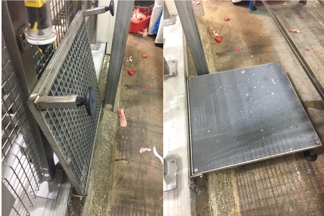
Fig. 25: Operator Platform – Raised / Lowered
