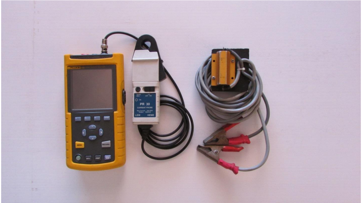
Photo 1: Fluke 43B Power Quality Analyser, Lem Heme PR30 Current Clamp and dummy load.
