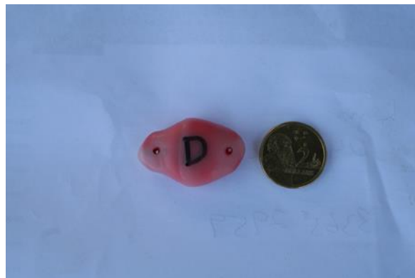
Figure 1. An IButton that has been coated in wax and is ready for implanting (note size relative to $2 coin)
