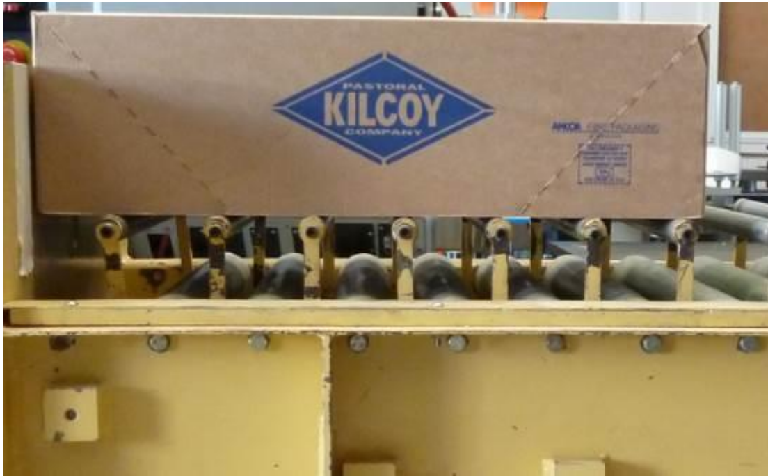
Fig.8 Roller conveyer designed and procured to accommodate the gripper
