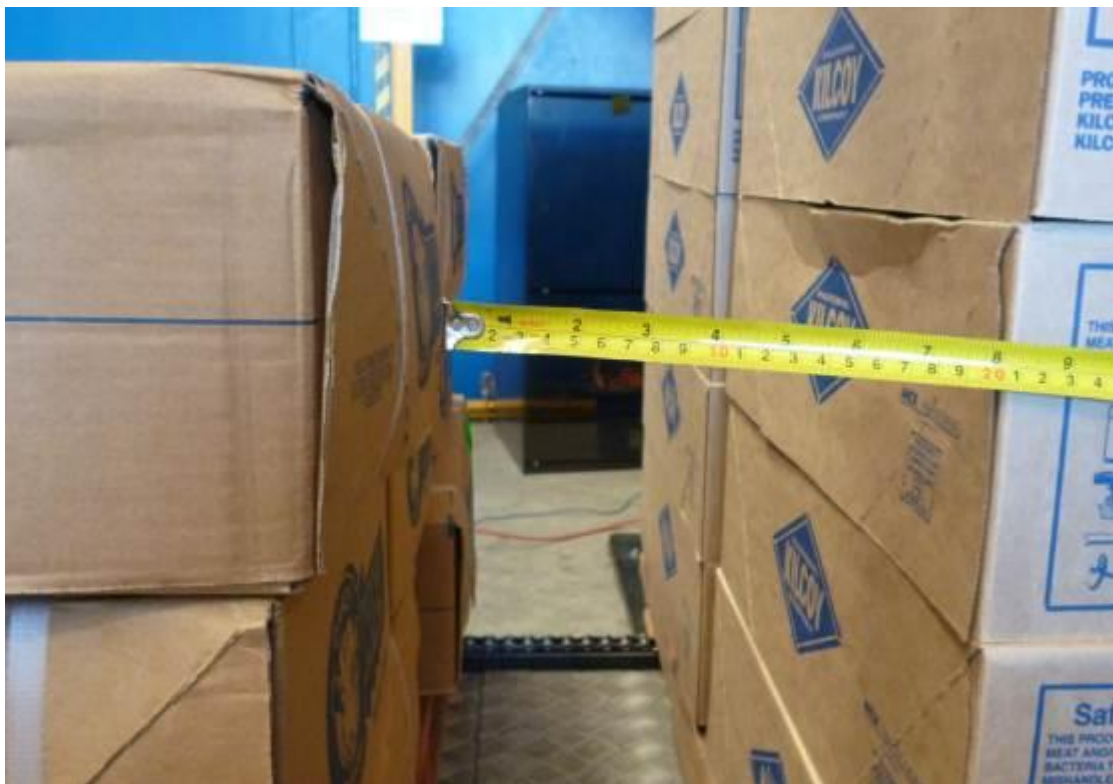
Fig.11 Distance between pallets and cartons
