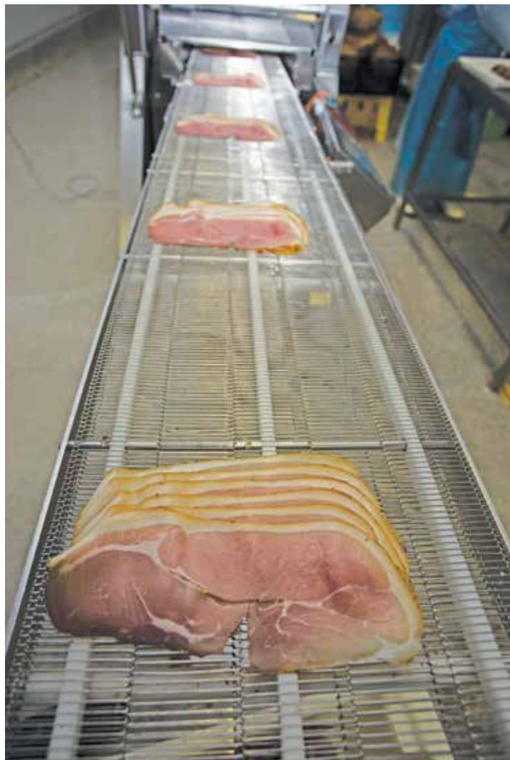
Figure 6.7 Conveyer belts are difficult to clean
