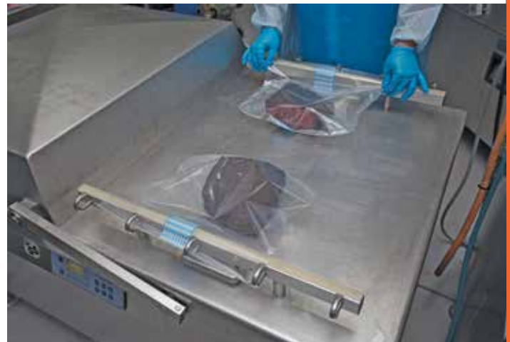
Figure 6.6 Manual vacuum sealer
