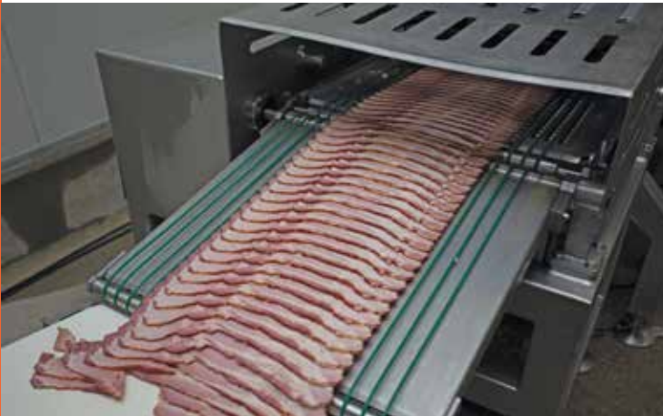
Figure 3.5 A slicing machine producing sliced bacon
