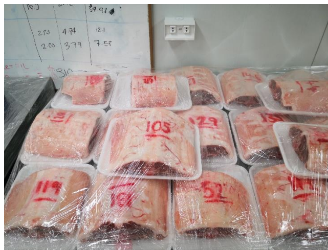
Figure 9 - A view of the selection of 30 mid-loins, individually wrapped on foam trays for easier moving between the chiller and CT scanner. From total sample size supplied by commercial abattoir the 30 mid-loins were selected to cover C-site fat depth variation.
