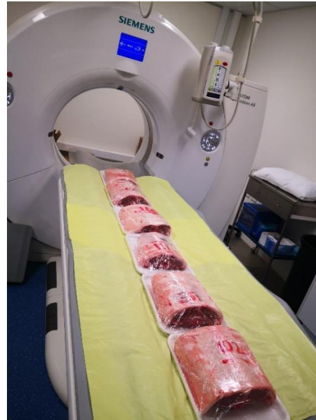
Figure 10 – Process of camera scanning and CT scanning of the mid-loins. Right: camera system scanning the mid-loins (two at a time), protective film is removed during scanning with the cameras, Left: CT scanner scanning 5 mid-loins at a time at a Medical Clinic in Armidale.
