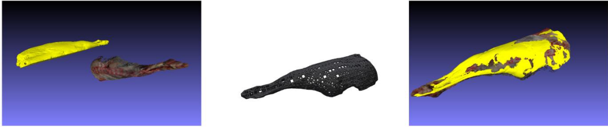
Figure 6 - Non-rigid alignment of CT mesh to depth reconstruction using embedded deformation, example shows a leg of lamb. (left) misaligned CT fat mesh shown in yellow and depth reconstruction, (middle) deformation graph of CT fat mesh, and (right) aligned CT fat mesh to depth reconstruction.
