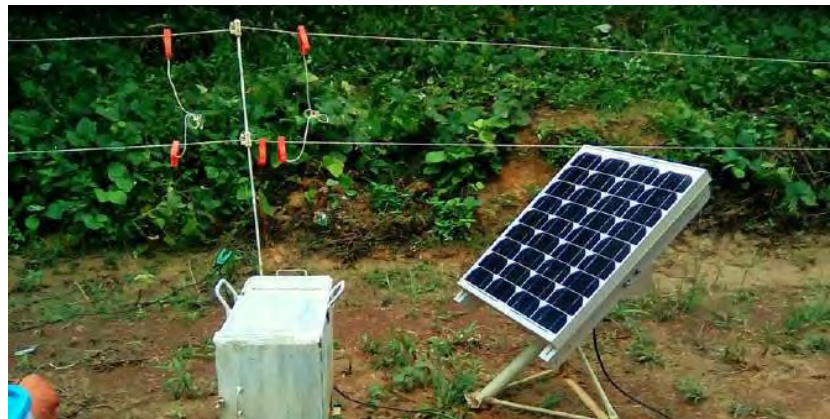
Portable electric fencing unit with solar panel
