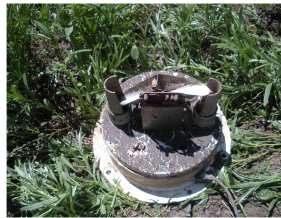
A rain gauge installed in a site subject to stormwater flows. The gauge was inundated and all components had to be replaced.
