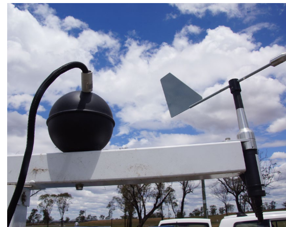
The black-globe sensor has a temperature probe inside to measure internal air temperature.
