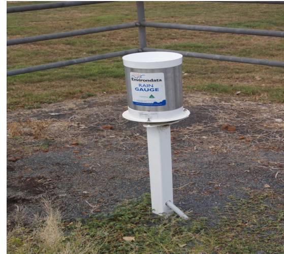
A rain gauge installed on a 600mm post to prevent flooding.
