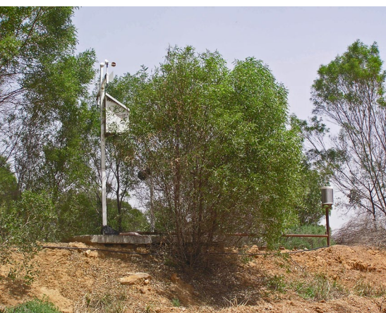
A less well sited AWS on a mound and shaded by close vegetation. Records would be unrepresentative of ambient conditions.
