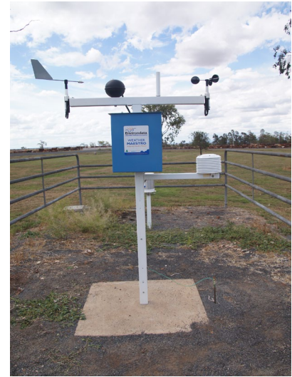
A typical AWS setup with sensors for wind direction and speed, and black globe solar radiation mounted on the cross-arm. Logger is mounted inside blue box.
