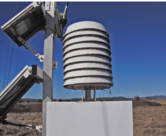
Spider webs and dust may affect the ventilation of humidity and temperature sensors within the screen.
