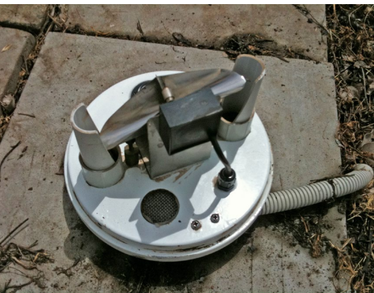
Tipping bucket rain gauge (pluviometer) with the cover removed – records rainfall total and intensity (mm/hr).
