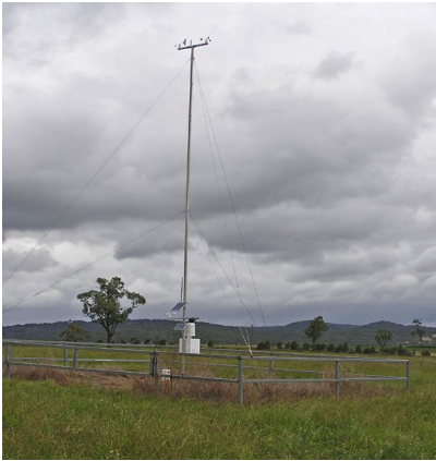
AWS mast with wind speed, wind direction and solar radiation at 10 metres, and other sensors at 2 m.
