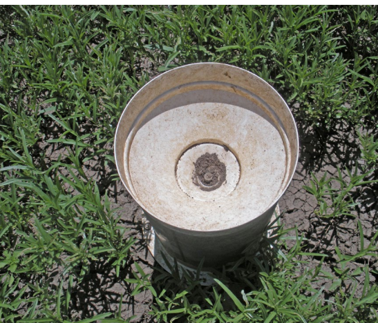
Dust – rain gauges need to be frequently inspected for dust accumulating in the bowl and cementing after heavy dew. Do not site AWS close to gravel roads.
