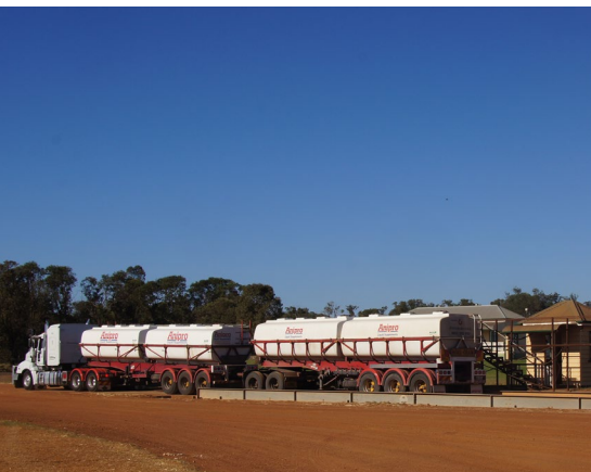
This weighbridge can take systems up to B-Doubles (in length), but a road-train would need to be weighed one trailer at a time.
